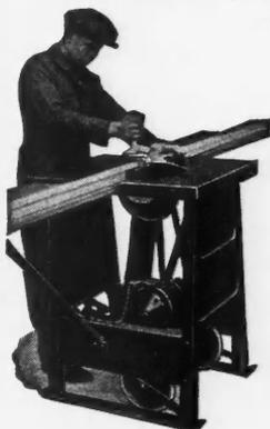
Here is a **POWERFUL, PORTABLE, CARPENTER SAWING MACHINE**. Will Cut Rafters, Studs, Stairhorses and Bridging; square long dimensions as fast as you can handle the lumber. For trimming sash, doors, screens, fitting casing and flooring.
