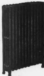
Four-tube Slenderized Radiator is less than 5 inches deep. Can be recessed and left open, or a Burnham Panel Front used, giving both radiant and convected heat.
