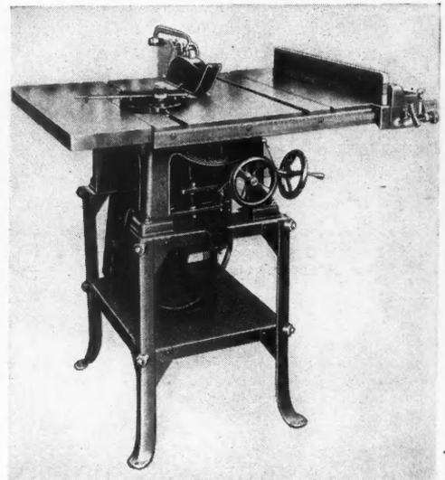
**TILTING** arbor saw on which lumber is always horizontal for any cut angle.
