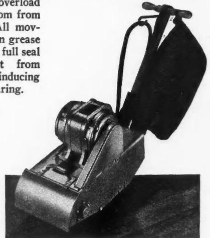
NEW floor sander has separate vacuum system used for dust collecting.
