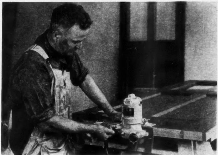
**PLANING** and fitting doors, sash and transoms are done quickly and inexpensively with this electric door plane. It will cut  $\frac{1}{8}$  inch off a 7-foot hardwood door in less than a minute.
