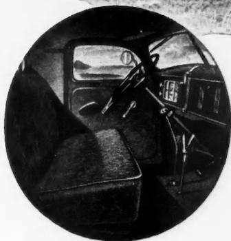
The **ALL-STEEL CAB** is a feature in every new International. The one-piece top, the sides, the back and cowl panels are welded into the complete cab frame. Rubber mountings wherever cushioning is needed. This is the roomy, well-appointed de luxe cab.
