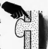
**RIVETED grip** formed as plaster is forced through its regularly spaced perforations to expand and form "mechanical rivets" on the back.
