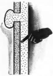
second, a **RIVETED** grip, formed as plaster is forced through its regularly spaced perforations to expand and form "mechanical rivets" on the back. That gives you walls that keep fresh looking, too, because they
