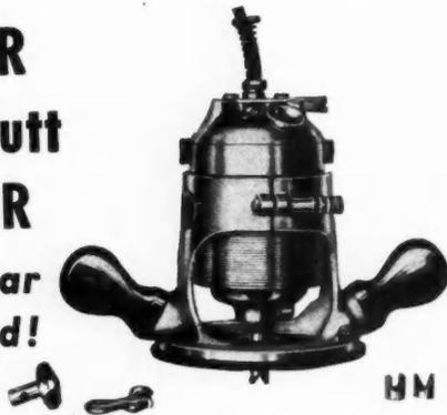
Mortises for butts 6 times faster than is possible by hand. Direct drive  $\frac{3}{8}$  H. P. motor runs at 18,000 R. P. M., cuts quickly, smoothly, accurately — leaves flat, even surface assuring perfect fit every time. High speed of cutters prevents tearing out wood between mortise and door edge. Used for all butt and lock face mortising.
