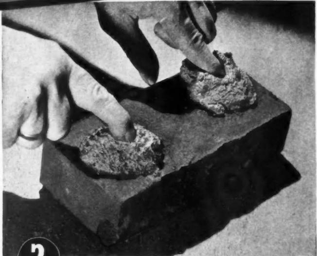
**2** Test each mortar. You will find that the Brixment mortar stays plastic *far longer* than the other mortar. This proves *greater water-retaining capacity*.
