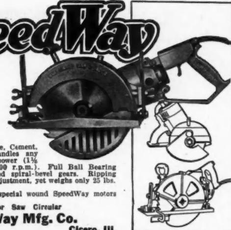
Cuts Wood, Tile, Marble, Cement, Slate and Gypsum, handles any and every job. More power (1 1/2 h.p.), more speed (4,600 r.p.m.). Full Ball Bearing construction. Guaranteed spiral-bevel gears. Ripping Guide, accurate bevel adjustment, yet weighs only 25 lbs. Grease twice a year. 5 other types all with special wound SpeedWay motors and new low prices.
