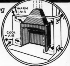
The Heatilator is a complete metal form around which any style of fireplace is correctly built. Eliminates many of the common causes of smoking.
