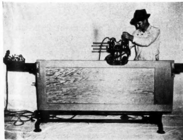
ABOVE at top: Contractor Zern's door fitting machine showing use of electric router. Lower view: Power mortiser in use; note electric planer at left end of machine, placed for immediate use.
