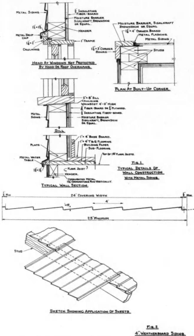
Fig. 1 shows typical details for wall construction with metal siding as developed by the Construction Division, Office of the Quartermaster General, including the various types of trimmings or flashings to be used in connection with its application to buildings such as water table, drip caps for windows and doors, side flashing for windows and doors, corner flashing for outside or inside corners and end wall flashing.
