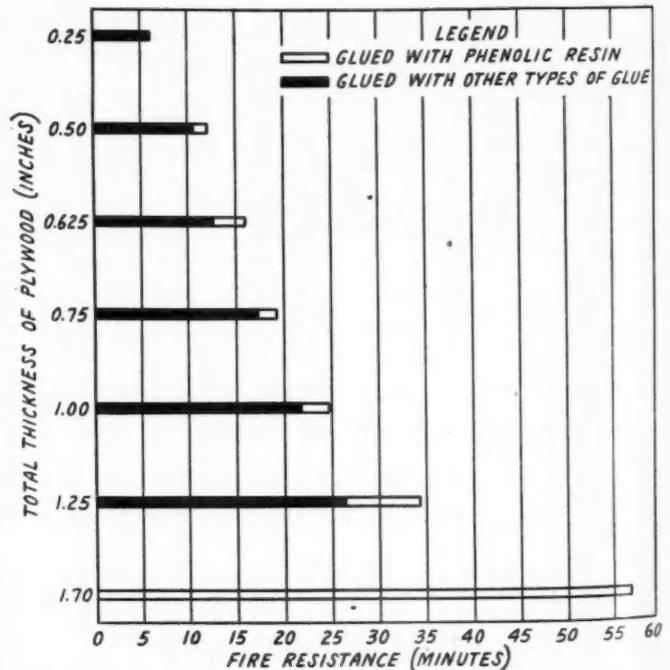
FIGURE 1.—Comparison of fire performance of phenolic-resin-glued plywood and plywood made with other glues.
