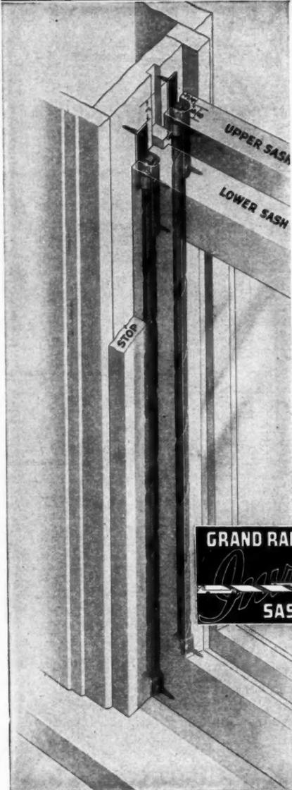
**NOTE:** Balance installation shows both sash lowered. Note that frames require no machining. No cuts in sash, except groove. No blocks required.
