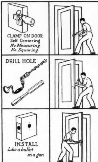
"Drill-Hole"—Dexter Bit-Guide directs the boring straight and true. Shallow mortise for face-plate and the door is ready.
