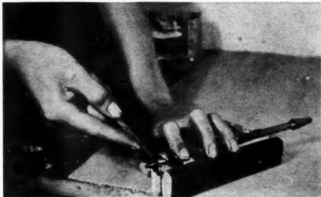
FILING auger bit made immovable by placing in wooden V-block.
