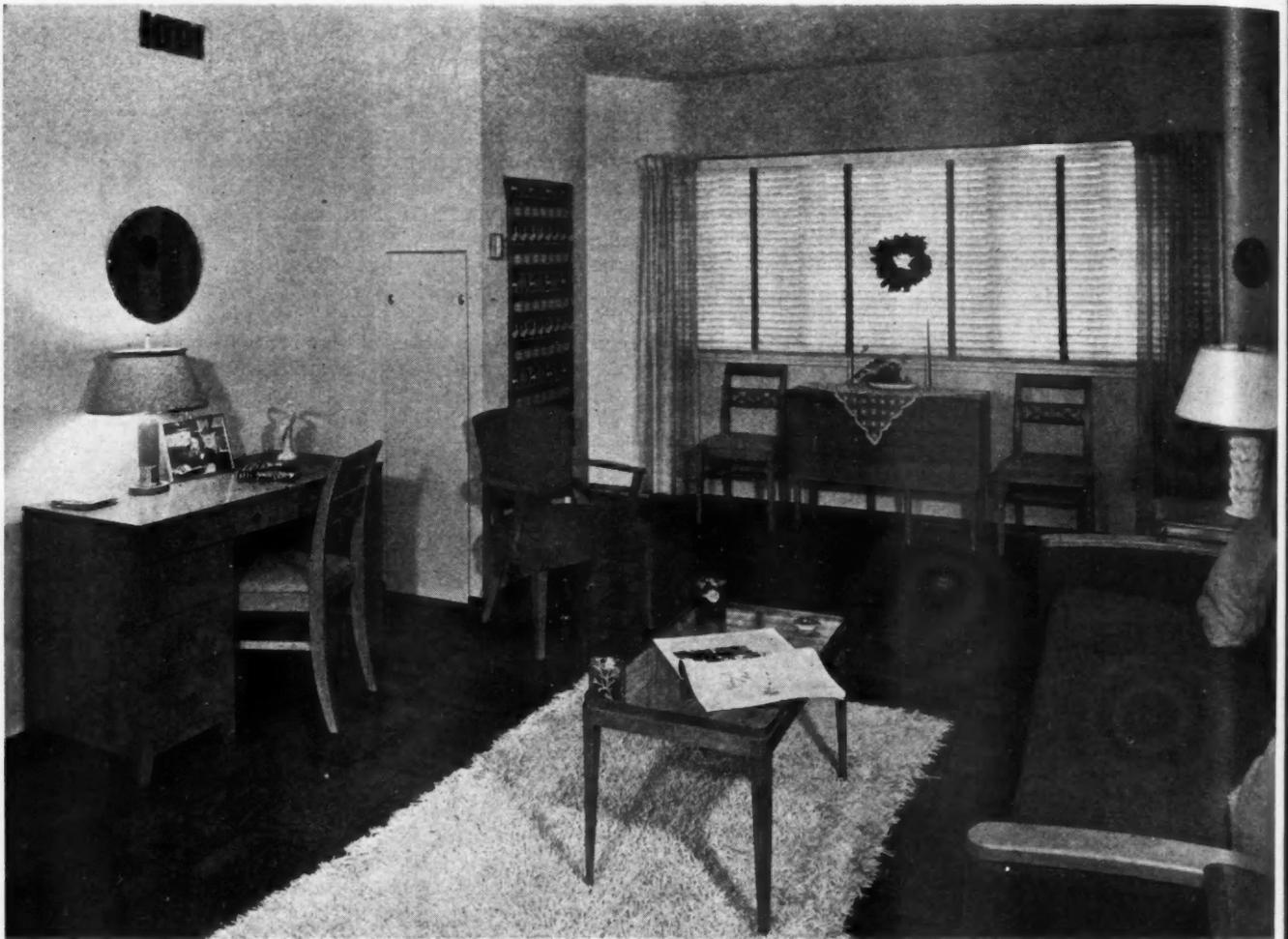
**TYPICAL Liebert apartment living room. Note at left, beyond desk the Janitrol Gas Fired Automatic Heating Unit with panel removed. When the plaster finish panel is in place only the inconspicuous flush locks differ from normal wall surface appearance. Heater chamber contains duct work, vent pipe, heater and heat controls.**
