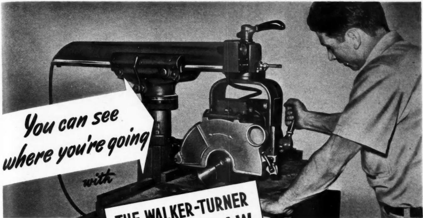
**YOU CAN** see where you are going when you use a **WALKER-TURNER RADIAL SAW**. The Ball Bearing Sliding Ram enables you to keep the work in full view at all times. Results—faster, more accurate work and greater safety.
