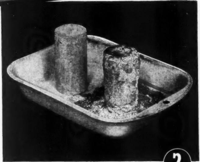
**1** Above: A cylinder of Brixment mortar (left) and a cylinder of mortar made with 50-50 cement and lime mortar (right). Both specimens were made at the same time, and subjected to exactly the same treatment. After curing for 30 days,  $\frac{1}{4}$ " of water
