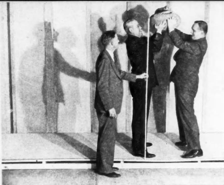
A 50-pound bag of sand dropped from a height of six feet fails to harm a Strong-Bilt Panel supported on centers 28 inches apart. Strong-Bilt Panels withstand impact blows up to 6 times that of boards with a mineral core.
