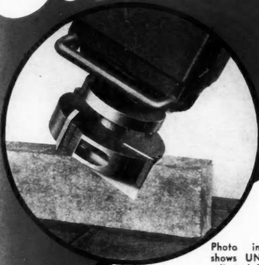
Photo in circle shows UNI-POINT adjusted for notch cutting operation, using a 4-knife countersunk cutterhead. Photo at right shows UNI-POINT set for compound miter cross-cut angle.
