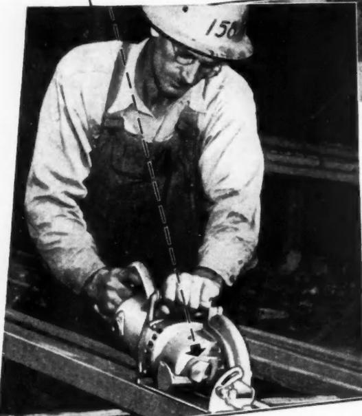
● Here's the high-powered SKILSAW you need for top-speed sawing on every cut up to 2<sup>5</sup>/<sub>8</sub> in. deep! Model "825" SKILSAW bevel-cuts 2 in. dressed—*or* rough—lumber at 45° ... sizes stone and concrete blocks ... cuts compositions and flat or corrugated metals. In fact, Model "825" makes practically every cut that's called for in construction!
