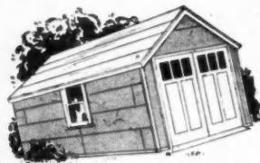
For all general buildings. Applied to studding, it combines siding, sheathing and insulation in one rigid, weather-resistant material... saves lumber, time, labor. Buff-tone or green mineral-surfaced exterior.  $\frac{7}{8}$ " thick—8' and 10' with square edges; 2' x 8' with T&G long edges.  $\frac{5}{8}$ " thick—4' x 8' with square edges.
