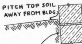
PUDDLE AND TAMP NEXT TO FOUNDATION USE INCH WATERPIPE TAMP DRILLED WITH AIR HOLES TO VENT POCKETS
