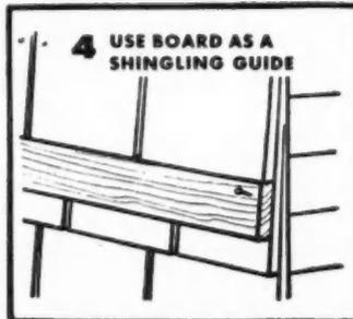
To provide drip-cap for rain-water. The top layer of shingles should project slightly below the other two. Shingle butts should not touch the ground.
