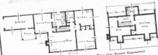
The plan (illustrated above) shows a home containing two rooms and bath, also a garage and porch. Provisions for future expansion of two rooms and bath on the second floor have been made.
