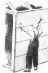
Celo-Rok Weather-Proof Sheathing is a fire-resistant gypsum board for use as sheathing or as composite sheathing and siding. Treated exterior requires no painting. 1/2" thick with T&G long edges; 1" thick with ship-lapped long edges. Sizes: 2 1/2' x 6', 8', 9' and 10'
