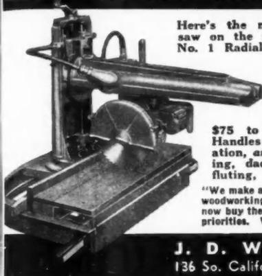
Here's the most practical contractor's saw on the market today—the Wallace No. 1 Radial Saw. With the exclusive Wallace Angulator, it cuts rafters complete with only ONE handling and without marking.
