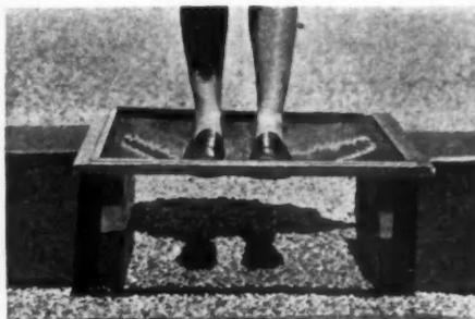
Plastic insect screen has six times the tensile strength of metal. Photo: Chicopee Mfg. Corp.
