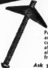
Paine Spring Wing Toggle Bolts take hold in hollow walls and provide sure, permanent support for hanging or securing fixtures. The two-piece toggle springs into place after insertion and will not pull out or work loose. Available in several head styles in standard bolt diameters from 1/4" to 1/2" in standard lengths.
