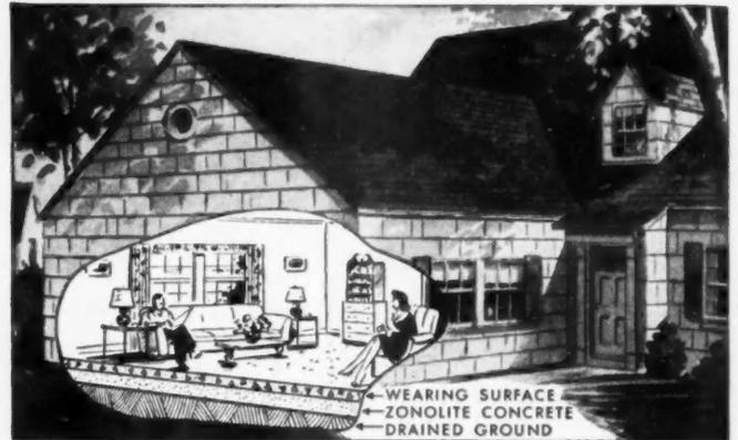
Warm, dry, permanent fire protecting floors are possible when Zonolite Insulating Concrete is used. It is adaptable for basement, ground or upper floors. Floors made from Zonolite Concrete are virtually free from dampness caused by condensation on warm, humid days. Can be placed directly on the ground. Proof against termites, vermin, rot and rodents. Ideal for basementless houses.
