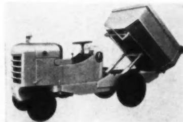
Its overall height is only 5 feet, 8 inches. The dump body is ideal for trucking sand, slag, castings, coal, cinders, gravel, ore, concrete or other bulk material. Built as a companion to the Payloader Shovel, the Payload Buggy matches it in capacity, compact size, speeds and operation. In addition, all main parts of the Buggy are interchangeable with those of the Shovel.
