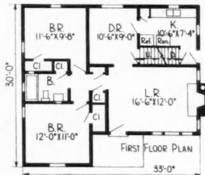
FIRST FLOOR plan of house above is shown at right. Both houses have forced warm air furnaces and plastered walls and ceilings. Landscaping is also provided
