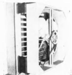
porates new features such as a fire-resistant sheet metal plenum, air-tight cushion seal, sealed bearings for all moving parts. The four-bladed fan is horizontally mounted with vertical air flow and belt drive. It is simple and easy to put in place in any ceiling. Only the clean lines of the automatic shutter are visible from below.
