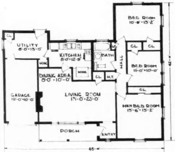
masonry placed on poured concrete trench walls 4 feet deep. A four-inch thick concrete mat is placed over the entire floor area. The mat is laid over a bed of cinders between vapor barriers. Asphalt tile cemented to concrete slab is used in all rooms. Steel casement sash are used in all window openings. Asphalt shingles cover the roof.
