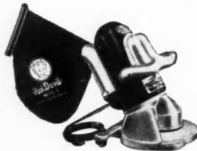
in to outlet. The edger weighs less than 35 pounds and is equipped with ball casters which will not mar the floor. The casters are adjustable.
