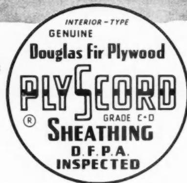
**PLYSCORD**—identified by this "grade-trade-mark"—is the sheathing grade of Interior-type Douglas fir plywood, manufactured in strict accordance with U. S. Commercial Standard CS45-48. It has a face panel of C veneer and a back panel of D veneer. Plys are bonded with highly water-resistant (but not waterproof) glues; the material will withstand occasional wetting such as might ordinarily be encountered during construction.
