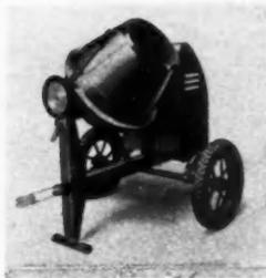
AB2970—Wonder "3" trailer mixer. Construction Machinery Co., Waterloo, Iowa. Half-bag capacity of any mix up to 1:2½:4. Electric welded frame, cantilever springs, pneumatic tires for high speed trailing. Engine, 1½ H.P., air-cooled, housed.
