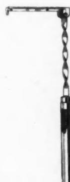
AB29157—Sash balance for counterbalancing double-hung windows. Unique Balance Co., Inc., 25 Bruckner Blvd., New York, N.Y. Comprised of a patented variable pitch spiral rod, coiled spring in metal tube, and metal fitting. Fastens directly to face of frame and bottom of sash. Easy to install. Assures trouble-free balance.
