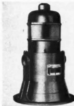
AB29136 — Self-priming centrifugal pump. Marlow Pumps, Ridgewood, N. J. The 10EV series have but one moving part. With 35 foot total head will deliver 34 gpm with 1/2-horsepower motor. Made in three sizes—1/5, 1/2, and 3/4 HP. Does a score of pumping jobs with minimum of attention. Positively self-cleaning.
