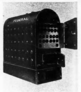
**AB29220**—Pictured is one of a new FD series of oil-fired, gas-fired and stoker-fired boilers. Federal Boiler Co. Inc., Midland Park, N.J. Designed for junior commercial use, steam ratings are 1,500, 1,800 and 2,200 square feet. Oil-fired bases are 12 inches high; stoker-fired, 16 inches high. Are S.B.I. rated.
