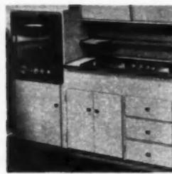
AB29245—Built-in cooking top, SU-3. Thermador Electrical Manufacturing Co., Los Angeles, Calif. Consists of three Thermo-Klean heating units, 35 inches long, 17 1/4 inches wide. Rough-in box, including drip trays, is 10 1/4 inches deep. Separate oven.
