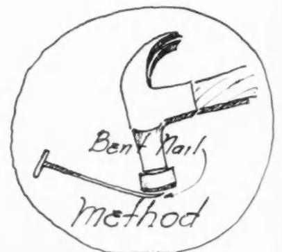
Greater strength is obtained through toe nailing when a slight crook is made at the point of the nail.
