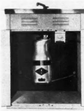
AB29366—Food waste disposer. In-Sink-Erator Mfg. Co., Racine, Wis. Can be installed on any sink having 3 1/2 to 4 1/2 inch opening. Requires only 9 1/2 inches from bottom of sink to wall outlet and 2-wire line to switch box of unit. Features reverse action that assures long trouble-free operation.
