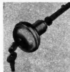
AB29275—Doorknob lock. La-belle Industries, Oconomowoc, Wis. Tumbler-type cylinder lock built into outer knob. Spins when locked. Cannot be jammed or sprung. When outer knob is locked, it remains locked even after door is opened from inside.
