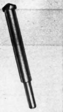
AB29368—Masonry drills. Kennametal, Inc., Latrobe, Pa. His high carbon steel shanks and a cutting blade of solid Kennametal. Blade has high resistance to wear and shock. Bit is used to drill tile, slate, stone, marble, brick, cement, plaster, asphalt, porcelain, micarta, and other nonmetallic materials.
