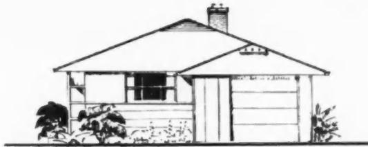
ALTERNATE design No. 1 is similar to basic house, except that garage and extended shelter replace small open porch. Orientation is the same. Plan below
