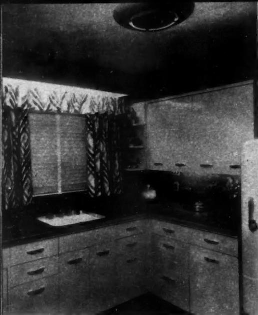
**PART** of kitchen in a \$17,000 house included in \$1,100 electrical package. Note provision for plug-in of small appliances and undercabinet lighting, which is supplied by portable fluorescent units that plug into convenient units
