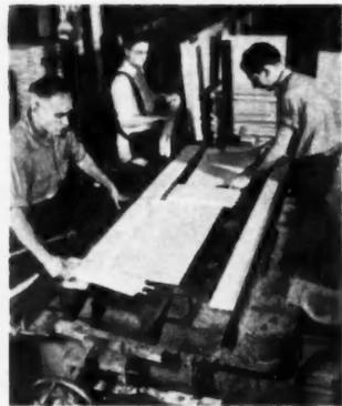
AB29107—Prespine panels. Curtis Companies, Inc., Clinton, Iowa. Door panels are cut and machined just like wood. Composed of sawdust mixed with a chemical compound, it comes out of heat press in large sheets resembling in color the natural wood. Material is used for all doors and kitchen cabinet panels.
