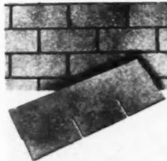
**AB29268**—Giant strip asphalt shingles. Johns-Manville, New York, N. Y. Felt base saturated and coated with refined asphalt. Granules imbedded in coating mineral, then second coat of asphalt and second coat of mineral granules are added next.
