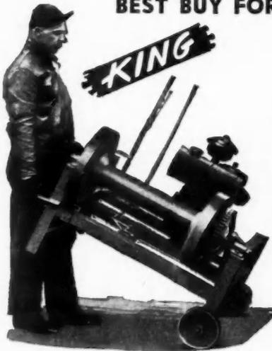
Four Models — 2 to 6 H.P.; air-cooled engine; easy on fuel. Handle like a barrel or bag truck. Two models specially designed for use with a derrick. Built to stand hard usage. Smooth, jerk-free operation. Simple to operate — no complicated parts.
