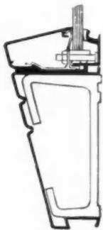
THE new Pittco De Luxe sill-sash combination gives the appearance of a single moulding combining the functions of sill and sash. Actually sill and sash are separate members designed to be used together in certain modern store fronts which require such a stylized assembly.
