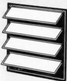
AB29105—Aluminum awning windows. Croft Steel Products, Inc., Jamestown, N.Y. Lemco, panoramic, solid-section, extruded aluminum windows of awning type. By a turn of the operator, the four vents tilt upward simultaneously, deflecting air currents to the ceiling. A flat screen is installed on interior.
