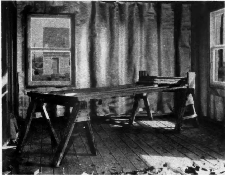
JIG, made at on-site shop, is used to speed up application of special sheathing-insulation material. Exact lengths of the material can be quickly cut, without necessity of measuring. Material feeds across jig table from roll on one end
