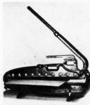
AB29154—Asbestos Siding and Shingle Cutter. Tri-States Building Materials Co., Ft. Worth, Texas. Equipped with two high-grade steel cutting blades 32 inches long. Has bolt adjustment for adjusting upper and lower blades. Cuts any thickness of asbestos siding or shingles. Weighs 37½ pounds; is 36½ inches long.
