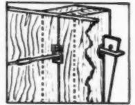
To strip forms, tap out wedges, remove bolts, then easily pull forms up or out without tools. Ties will break back inside wall, 1" from the surface by twisting loop 1/2 turn.
