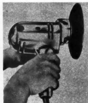
**AB29203—Portable electric tool.** The D-6. Porter-Cable Machine Co., Syracuse, N. Y. A 5-in-1 tool that will sand, polish, cut, drill, and stir paint by simple attachment changes. Will drill wood, plastics and compositions up to 1/8 inch hole, metals up to 1/4 inch hole. Weight 5 pounds 13 ounces. Used overhead or vertically.
