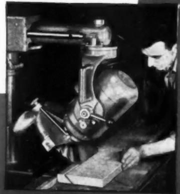
Straight ripping or bevel ripping is easy with Radial SKIL Saw. The operator simply slides the material along the rip fence for accurate cuts.
