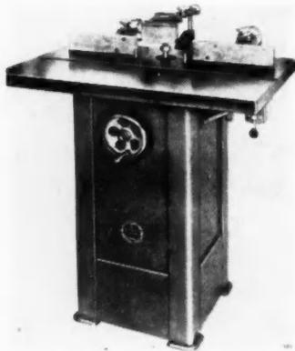
Shaper has three inch vertical spindle travel, with bearing assembly moving as a unit. Elevating is controlled by hand wheel and graduated dial; independently adjustable guides are controlled by hand wheels. Motors are 1 HP single phase or 1 1/2 HP three phase. Walker-Turner Div., Kearney and Trecker Corp., Plainfield, N.J.
