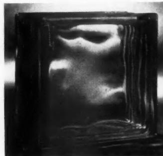
other places where decorative effects are desired. Random effect is achieved in production by use of several slightly dissimilar molds to form two halves of block, then using different combinations of halves. Designated as Insulux Glass Block No. 331. American Structural Products Co., Toledo, Ohio.
