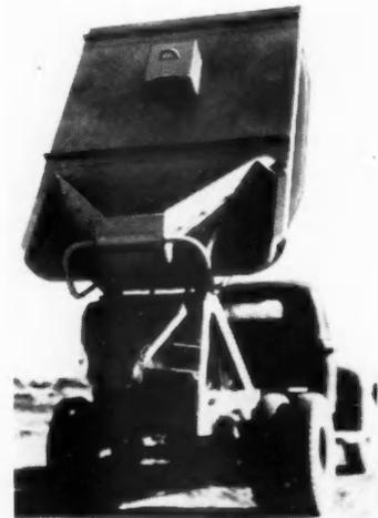
ready-mix lime mortar. Has four cubic yard capacity. High discharge point allows use of long, fully adjustable chute. Vertical dumping angle and rounded interior corners aid clean discharge. Dumpcrete Div., Maxon Construction Co., 131 N. Ludlow St., Dayton, Ohio.
