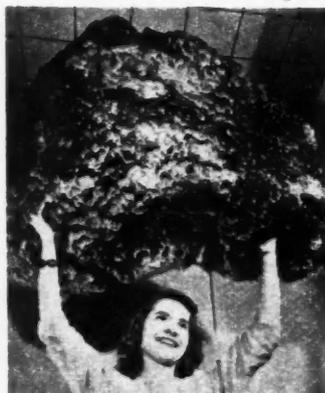
10 to 20 times less than pie meringue, is resistant to fire, moisture, fungus growth, insects. Liquid resin can be foamed into place at site of use. Westinghouse Electric Corp., 306 Fourth Ave., Pittsburgh 30, Pa.
