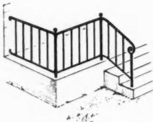
construction throughout. Handrail is  $\frac{3}{8}$  inch x  $1\frac{1}{4}$  inch bar stock terminating in a hand-wrought scroll finish at newel post. Pickets are one-half inch square. Horizontal straight rail sections are manufactured for use in conjunction with 7x12' rail section. Railing sections bolt together, using intermediate newel posts; will fit a number of masonry conditions. R. G. Coffman Co., Inc., 2809 N. Orange Ave., Orlando, Fla.
