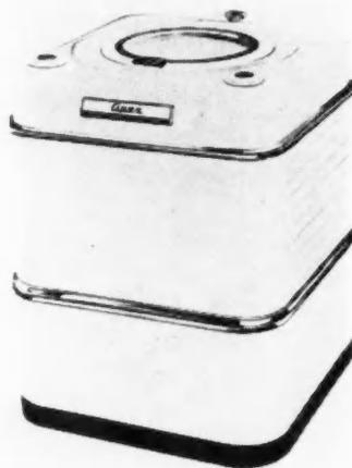
ished stainless steel. Electric automatic timer controls wash-rinse-dry-fluff cycle. Two dial settings for wash—hot (tank temperature) and warm, 100 degrees F. Motor is heavy duty 110 volt, 60 cycle AC. Dimensions: 36 inches high, 26 1/4 inches deep, 26 inches wide. Apex Electrical Manufacturing Co., Cleveland, Ohio.
