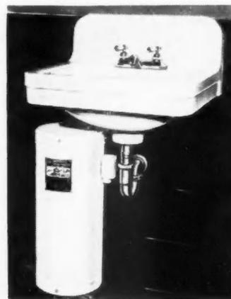
tached to wall next to basin. Has Fibreglas wool insulation, spreader tube, blanket type heating elements. Models have capacities from one to five gallons, with 110 volt AC current. Widths from 8 inches to 13 1/4 inches; heights from 19 1/2 inches to 35 inches. Barton Products Inc., Defiance, Ohio.
