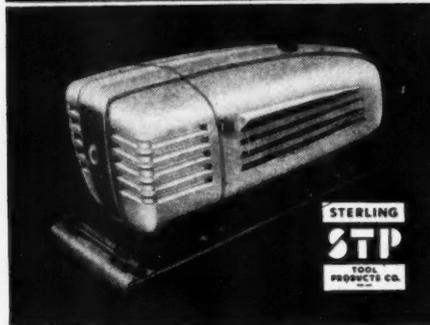
New design, new construction, new power... at low cost! The new Century Sander provides the utmost in speed, quality and dependable service. Specifications: Series wound, Universal 115 or 230 volt, 0 to 60 cycles (AC-DC) type motor (which cannot be stalled). Die cast, aluminum alloy housing. Grease packed anti-friction bearings.
