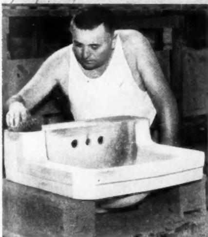
John Bandies is a veteran of the ceramics industry with 34 years' experience. As a caster, he checks each fixture as it is removed from the mold. He carefully sponges the unit, smoothing the edges and flat surfaces, and looking for defects. After inspection, his number, 102, is stamped into the fixture and it is ready for the drier.
