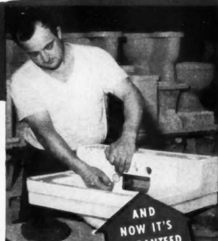
John Rosko, a Final Inspector, has been checking chinaware for over 10 years. Rosko carefully inspects each unit as it comes out of the automatic, continuous-fire kiln. When his detailed inspection is completed and the fixture passes, it is classed as 1st quality ware. His inspector's seal and the Richmond guarantee are attached. The unit is now ready for shipment.
