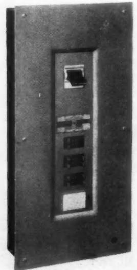
16 and 20 circuit combinations for either three or four wire service. Incorporates thermal-magnetic circuit breaker units that plug in on cylindrical bus bars and are interchangeable with those of NMO panel-board. Plug-in feature simplifies changes or additions of circuits when load increases are necessary. Underwriters' approved. Square D Co., 6060 Rivard St., Detroit 11, Mich.
