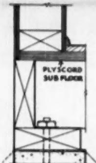
SECTION of an exterior wall running across the joists. First joist is cut  $\frac{5}{16}$ -inch outside of stud line to provide for  $\frac{3}{16}$ -inch plywood panel. This simplifies use of standard 4x8 foot sheathing panels, applied either vertically or horizontally
