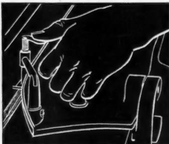
**Handling narrow strips**—This narrow strips can be planed down to small dimensions by feeding strip between the fence and curved lower edge of the Dual Purpose Guard using thumb hold down device.
