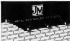
**WITH BRICK VENEER:** In this construction the brick ties are simply nailed through the Johns-Manville Weathertite Sheathing and into the studding.
