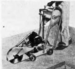
Four wheel Model CHD cart quickly converts Clipper masonry saws to Clipper concrete saws. Triple duty use can be obtained with gasoline or electric powered units. Standard Model HD saws are used to cut brick, tile, stone or any masonry material that can be placed on its conveyor cart. Now with convertible design cutting head can be positioned in CHD cart to saw concrete floors, walks and streets. Clipper Manufacturing Co., Dept. AB, 2800 Warwick, Kansas City, Mo.
