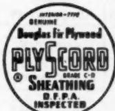
PLYSCORD® is the sheathing grade of interior-type Douglas fir plywood, banded with highly moisture-resistant (but NOT waterproof) glues which will withstand occasional wetting such as might be encountered during construction. An unsanded panel for wall and roof sheathing, subflooring, backing, bracing and one-use concrete forms.
