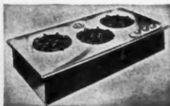
**"IN-A-TOP"** 3-Burner Drop-in with plated surface fits into a counter top or sink cabinet by providing opening of 18-1/2" x 33-5/8". Individual drip rings may be removed easily for quick cleaning. Also available with 4 burners.
