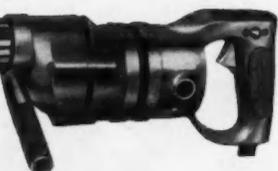
For straight drilling, S-412 1/2" HOLE-SHOOTER (above) has a chuck speed of 450 R.P.M. With the 2-speed "Right-Angle Drive" attachment, speeds are 300 R.P.M. or 675 R.P.M.
