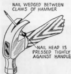
method which eliminates the use of grooving or rubber bands. All one has to do is simply to slide the nail between the claws of the hammer with the head of the nail pressed tightly against the handle.
