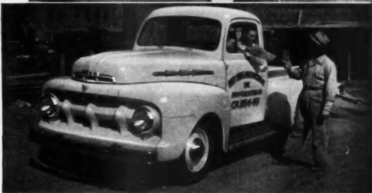
This 6½-ft. Ford Pickup for '51 is also a great favorite with contractors. Body has sturdy wood floor. Low 2-ft. loading height. Steering column gearshift. Cab rear window 3½-ft.
