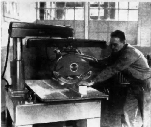
**RADIAL SAW** This new 16" Delta Radial Saw cuts through the entire 360° at every conceivable angle. All cuts are made above the work table, in clear view. For miter capacity and extraordinary versatility, this saw truly has no equal. Also available on 8", 10", 12" and 14" models.
