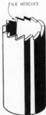
To make an improvised star drill take a piece of pipe of the required diameter and file notches in one end with a saw file. This can be used in a pinch when a star drill is not available.—John Menkveld, Grand Rapids, Mich.
