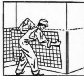
**FIG. 8**—Cut the hardboard with a fine tooth crosscut saw and sand edges before fitting and installing. Bevel back edge of board slightly for perfect fit. Scored edges of the board should always be kept to the top and right
