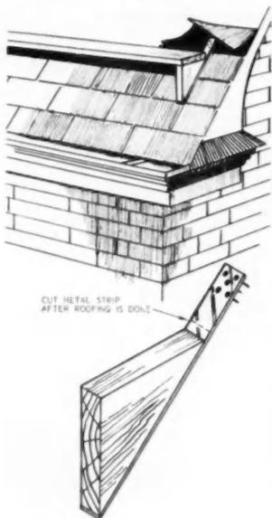
To make an effective shingling bracket take the blocks that are cut out of stair stringers and nail a strip of heavy gauge sheet iron on one side. Nail the top of the metal strip under the shingles and use a 2x6 inch plank on top of wood blocks for a toe hold. The exposed portion of sheet metal is cut off at the edge of shingles when roofing is done.—John Menkveld, Grand Rapids, Mich.
