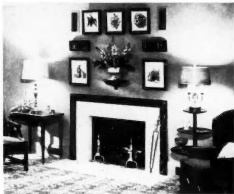
**TYPICAL** attractive fireplace in home of modern design utilizing a metal fireplace unit with hot air grilles located in wall near ceiling and cold air return grilles in baseboard at either side
