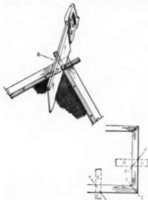
Nail together screen mouldings shown at B with ends projecting. Saw through mouldings at B with thin saw. Mouldings of various widths may be mitered by sawing on a line through C-C. Window screens with a three-inch bottom rail can be cut this way, or as shown in E-E or C-C.—M. J. Hiland, Lansing, Ill.
