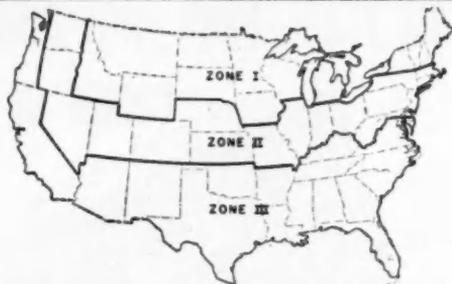
FIGURE 6.—Condensation zones.—Zone I roughly includes the areas with design temperatures  $-20^{\circ}$  F. and colder; zone II  $0^{\circ}$  to  $-10^{\circ}$  F.; and zone III areas warmer than  $0^{\circ}$  F.
