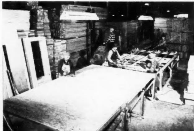
**PRODUCTION LINE** for roof panels. Plywood sheathing covers the rafters and serves as the base for roofing paper and asphalt shingles which will be applied at the site
