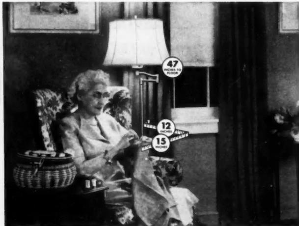
Typical Light Conditioning recipe built around a specific seeing task. It shows by actual measurement how to provide the right lighting for sewing.
