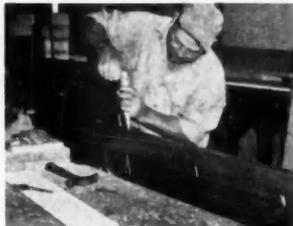
**WORKMAN USING A POWER SCREW-DRIVER** to fasten hinge butts in previously routed mortises. Power tools cut costs in finishing operations
