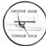
Complete wrap-around support—the Nu-Wood Clip completely "wraps" tile tongue and groove edges with metal—supporting both tiles. Thus, ceiling tiles stay in place when applied with Nu-Wood Clips, assuring a level surface.
