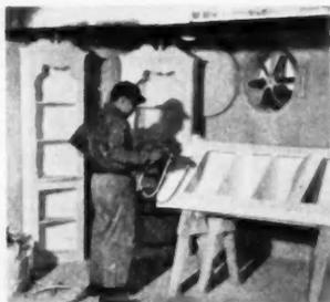
A POWER SPRAY UNIT, fed from a pressure tank, is used in the shop for spraying doors, cabinets, and bookshelves. Note exhaust fan for worker protection against fumes
