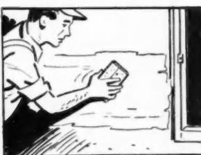
**5** Sandpaper surface lightly after cement has dried to remove any rough spots
