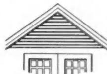
On new construction it costs little to include exhaust openings to handle attic ventilation. These may be gable louvers or porch, soffit or basement exhausts, depending on the design of the house.
