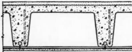
**METAL LATH ATTACHED TO CONCRETE JOISTS.** Hangers for attaching metal lath directly to the underside of concrete ribs approximately 25 inches on center should be placed in ribs before concrete is poured. They should be hook, loop or hairpin type, not less than 14 gauge galvanized annealed wire when twisted as in tie wire and not less than 10 gauge galvanized wire when struck over to support the lath. Space not more than five inches apart
