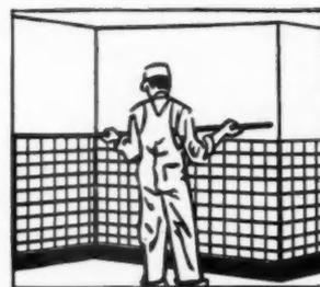
**FIG. 11**—After wainscot has been installed, apply cap and base mouldings by cementing, by nailing, or by both
