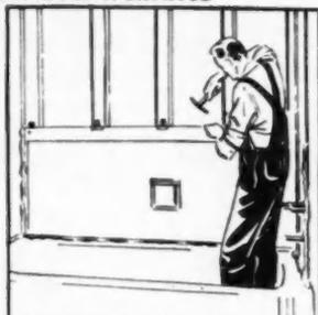
**FIG. 23**—Set the plate at the back of the tub first. Then merely nail through plasterboard flanges and use the special clips supplied for this type of installation
