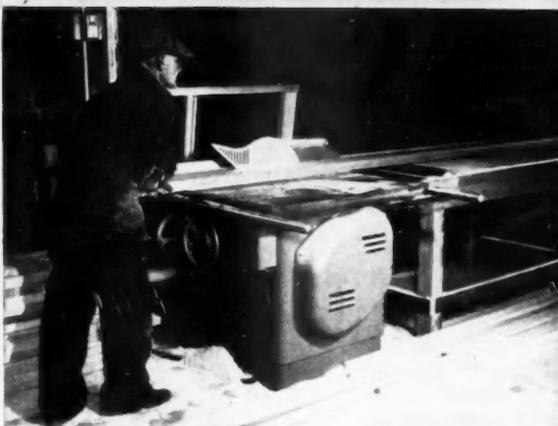
**CIRCULAR SAW** Mass production ripping is exceedingly simple on this massive, rugged, big-capacity Delta 12" tilting arbor saw. Its accuracy is built-in for long years of usefulness. For dependable performance and operating economy, there's nothing finer. Also available in 10" and 8" models.
