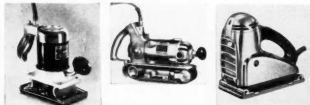
**THREE HAND SANDERS FOR FINISHING OPERATIONS.** The unit at left operates with a reciprocating motion, using sheet sandpaper. Center is belt type, for larger areas. Right is an orbital type, in which the abrasive is moved in a circular motion
