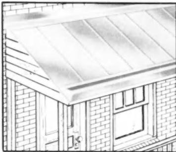
Porch roof—vertical and horizontal seams are flat locked.
