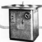
Whitney 510 SHAPER — Belted, motor drive. Table, 36" x 31". Vertical adjustment of spindle, 3 1/2". Detachable spindle top.
