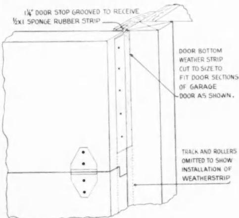
Sketch above indicates two methods of weatherstripping upward-acting garage doors. This makes for a better and tighter fit and also cuts down excess friction from stopping on face of door.—Paul R. Kersten, Greensbury, Pa.
