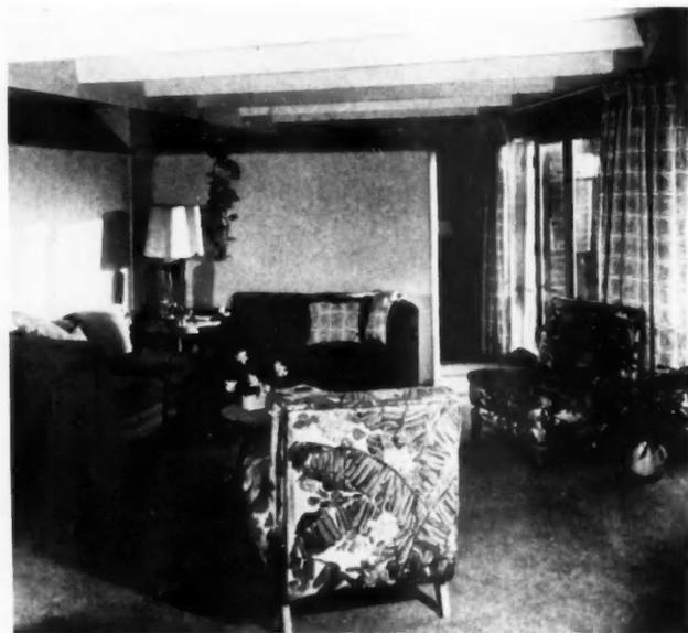
Finished product. Ceiling projections are the exposed steel box joists. Interior walls are solid plaster partitions.
