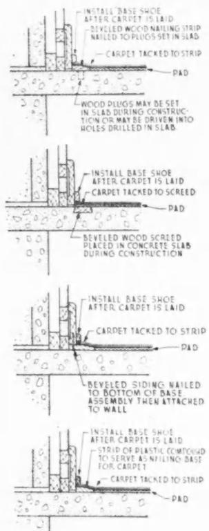
Methods commonly used for attaching wall-to-wall carpeting to concrete subfloors
