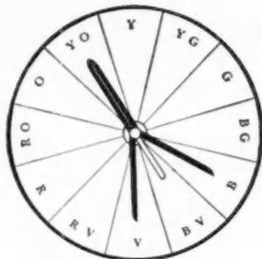
**FIG. 5—SPLIT COMPLEMENT,** for a 3-color plan. Colors on either side of the complementary color provide harmonious contrast. Proper proportions of each color used would determine the success of the decorating scheme.
