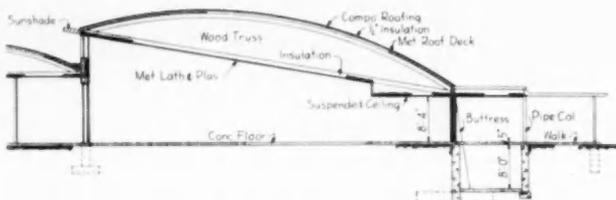
By tilting the large trusses of the roof of the Jewel Tea store, the store is made to seem larger, actually is lighter, and an interesting accent is added to the center's architectural mass. The drawing of this construction shows how the entrance to the store is kept low, encouraging the feeling of intimacy which food merchants consider desirable in a customer entering the store
