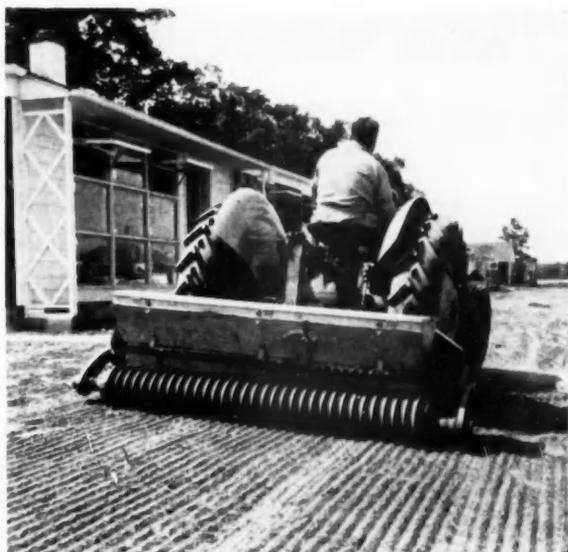
Seeding operation uses a Brillion seeding attachment. The farm machine combines seeding, fertilizing, and rolling in one pass
