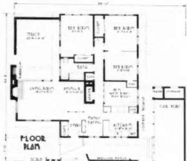
Floor plan indicates that space of 1,285 square feet is divided into five to eight rooms, depending on how you count. Deep carport has solid outer walls, plus enclosed storage areas in rear
