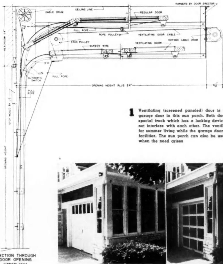
**I** Ventilating (screened paneled) door is used with a standard garage door in this sun porch. Both doors are operated on a special track which has a locking device so that the doors do not interfere with each other. The ventilating unit is available for summer living while the garage door affords winter storage facilities. The sun porch can also be used as an extra garage when the need arises
