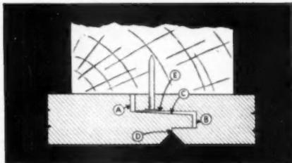
**Cross section of J-M Lightning Joint.** Notice the spaces at A and B to provide for expansion and contraction... the tapered edge of the tongue C to facilitate joining... the square-corner edge D to make alignment easier... the large nailing area E for concealed nailing or stapling.
