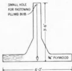
A simple level may be made from  $\frac{3}{8}$ -inch plywood. A carpenter's square is used in marking a center line as guide for plumb bob. Before marking, reverse position of level to check line. A small hole is bored near top of line for fastening plumb bob.—Arthur N. Nelson, Kansas City, Mo.
