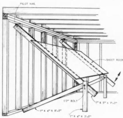
The sketch, left, shows a method for applying dry wall panels on a ceiling with the aid of a simple jig.
