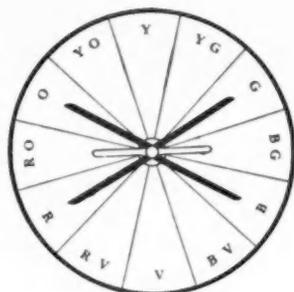
**FIG. 6—DOUBLE COMPLEMENT,** for a 4-color plan. Two sets of complementary colors are used. Remember that neutral colors may also be used with any color or combination. "Monochromatic" schemes can be worked out effectively in tints and shades of a single color.
