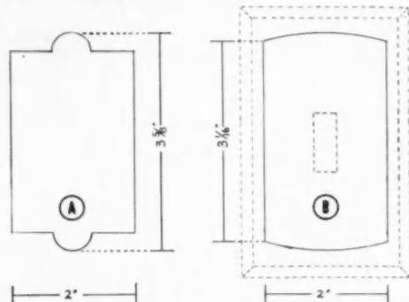
Instead of trying to cut holes in gypsum board to fit convenience outlet boxes as indicated on sketch at (A), it will be easier and quicker to cut holes for the same as shown at (B). The finish plates are  $2\frac{3}{4} \times 4\frac{1}{2}$  inches so they will cover.—J. G. Caldwell, San Mateo, Calif.
