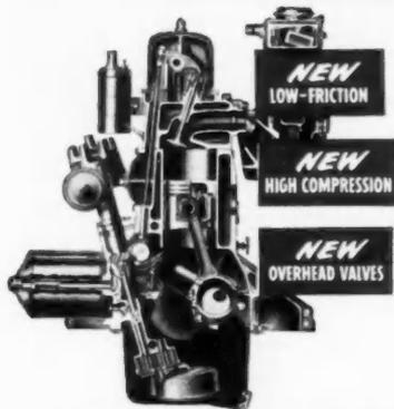
This new Ford 101-h.p. Cost Clipper Six is one of the best proved truck engines ever introduced. It had 50,000 dynamometer test-hours and over 500,000 vehicle test-miles.
