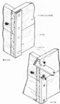
When form nails are not available for setting up forms, then common nails and pine plaster lath may be used. Lath are ripped off when stripping forms. This leaves nails free to pull.—W. A. Woodard, Volga, So. Dak.
