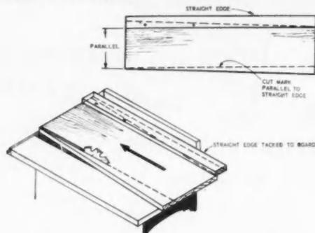
Mark the board on which the work is to be done. Tack straightedge parallel to mark with the straightedge guiding work along the rip fence.—Werner Kraatz, Santa Cruz, Calif.
