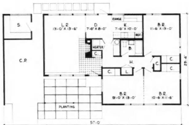
Floor area is 1078 square feet. Ten-inch boards with 3-inch battens give sharp vertical accents to a horizontal design. Roof pitch is 2¼ inches to 12 inches. Chimney is masonry. Obscure glass is used in skylight which serves halls
