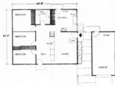
The houses take full advantage of the open planning principle. There is no clear-cut separation of areas except for the bedrooms and the bathroom. The kitchen is concealed from the living room only by a baffle partition. The play area—an important innovation—is defined by a storage partition which stops short of the ceiling.
