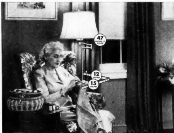
Typical Light Conditioning recipe built around a specific seeing task. It shows by actual measurement how to provide the right lighting for sewing.
