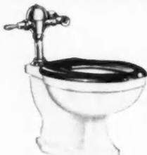
Sanus E-5910-V—Vitreous China, Syphon-Jet Closet, with elongated rim. 1½" top inlet for flush valve, as specified. Projection from wall, 28¼". (With round front, projection from wall, 26¼".)
