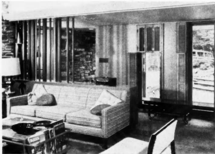
Open plan utilizes random-width dowels with brass light fixtures suspended among them and a long, low cabinet to separate living room from gallery opposite main entrance. Plate glass doors off gallery are also fitted with roller screens and hinged shutters. Floor tile of gallery matches that of terrace, is flush with height of carpet
