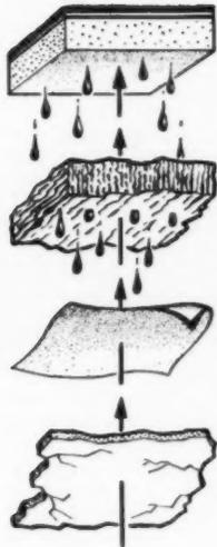
Vapor flows through Plaster, through Asphalt, into ordinary insulation and condenses. Also condenses on inner surface of cold outer walls and roofs.
