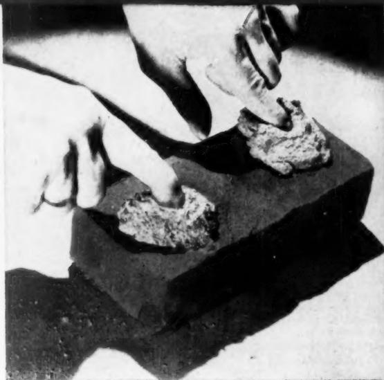
each dab. The one that stays plastic longest will be the one having the highest water-retention. Try this with Brixment mortar!
