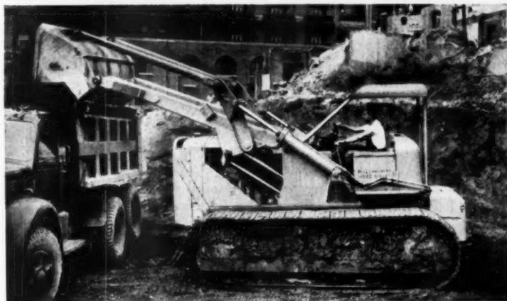
Excavating dirt and rubble from old building and loading to trucks is one of many jobs this Allis-Chalmers HD-20G tractor shovel handles fast because of its 175 net engine hp., easy maneuvering ability and big 4-yd. bucket capacity. Working on large housing projects, the 61,600-lb. HD-20G's economically dig a basement an hour in any weather, clear out trees, move big rocks.
