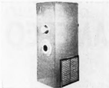
**AB13272—OIL-FIRED FURNACE**—Kaustine Co., Inc., Dept. AB, Perry, N. Y. The "Jersey 75" unit is offered as being suitable to cover the heating requirements of the small house. It has a capacity of 75,000 B.T.U.'s at the bonnet, and covers only 3½ square feet of floor space. The unit incorporates a new "air-way" combustion chamber with chrome steel fire pot liner and aluminum foil inner insulation. The furnace measures 21 inches wide, 24 inches deep and 60 inches high.
