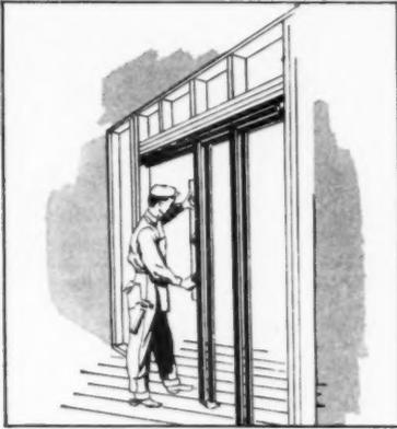
It takes a carpenter several hours to frame-up a rough opening, and install hardware for a disappearing door. But at best, he can't guarantee the job, simply because warpage often ruins the installation. Exposed to the ravages of heat and humidity, horizontal wood members—and the door itself—tend to buckle and bind.
