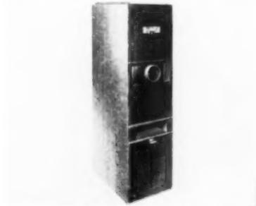
**AB13270—GAS FURNACE**—Armstrong Furnace Co., Dept. AB, 851 W. Third Ave., Columbus 8, Ohio. A new 65,000 B.T.U. gas-fired counterflow furnace is offered this year by Armstrong. It has been designed particularly for the small basementless one-floor house. Return air is brought in from the top of the unit, and warm air is discharged through the bottom into an under-the-floor heat distribution system. Hence it is ideally suited for use in perimeter heating. Size is 17x26x62 1/2 inches.
