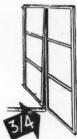
Ventilator should toe out at bottom— $\frac{3}{4}$ " for each light high.
