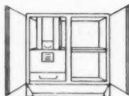
**RANGE HOOD** fits over cooking area on bottom of cabinet. Trade-Wind ventilating fan operates inside cabinet.
