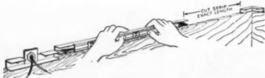
Place "Plug-in" Strip against the wall in proper position on the baseboard. A downward thrust on the Strip slides it firmly into place. The screw holes in each end of the base may also be used for mounting.
