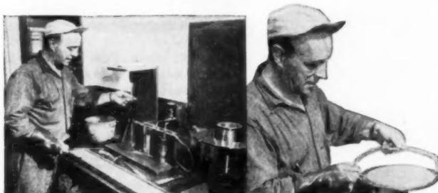
\* High Water Retention is the basis of workability, plasticity and bond. In Lone Star Research Laboratory, this standard test simulates sucking action of brick. Suction is applied to mortar for one minute. Difference in flow of mortar, before and after test, indicates plasticity and water retention. Write for new Masonry Booklet—address Lone Star Cement Corporation, 100 Park Ave., New York 17—or nearest office, below.
