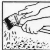
Spattering is done after the floor has been painted a solid color and allowed to dry. Have the brush well filled with the contrasting color selected, and strike the brush sharply against a stick or piece of iron pipe held in the other hand. Small spatters are made with less paint in the brush and by striking the brush against the stick held about one foot from the floor. Make large spatters with a brush full of paint and by holding the stick about three feet from the floor.
