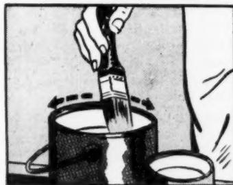
Dip it in about ⅓ the bristle-length. Tap gently on sides of can to "settle" the paint into the brush. Never scrape on rim of can. Always start with a clean brush.
