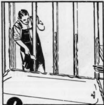
**1** After tub has been levelled, place roll of mastic around rim for waterproofing. Also, butter studs with mastic before setting glass panels.
