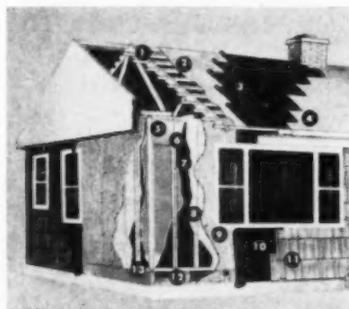
Component parts of prefabricated home at left include: (1) Truss supports; (2) Roof sheathing; (3) Roofing paper (4) Asphalt shingles; (5) Gypsum board ceiling; (6) Wall framing stud; (7) Upson board with moisture barrier; (8) Fiberglass insulation; (9) Plywood sheathing; (10) Asphalt barrier; (11) Shakes or siding; (12) Box beams; and (13) Flooring
