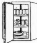
**REVOLVING CORNER WALL UNIT** is similar in design to the base unit shown left. Also saves space ordinarily wasted.
