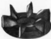
Heart of the Ceil-N-Wall. Impeller is designed to deliver exceptionally high air volume through long ducts and elbows and against high static pressure. Impeller disc and baffle plate prevent air recirculation. Extremely quiet in operation.
