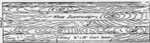
**CANT STRIP:** Formed after deck has been prepared by applying 1/4x1 1/2-inch wood lath over wood sheathing along edge of eaves
