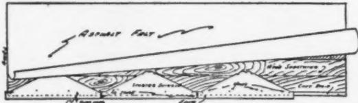
**STARTER COURSE:** Lift up felt along eave and apply a full size starter shingle to overhang rake and eave 1-inch. Use four nails per shingle, 1 1/4-inch for new work, 2-inch for re-roofing. Next starter goes parallel to eave with 1/16-inch space between vertical edges of shingles
