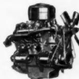
Overhead valve, 101-h.p. *Cost Clipper* Six, 145- and 155-h.p. *Cargo King* V-8's—cut down on friction power waste, save gasoline. Also, 106-h.p. Truck V-8 and 112-h.p. Big Six.
