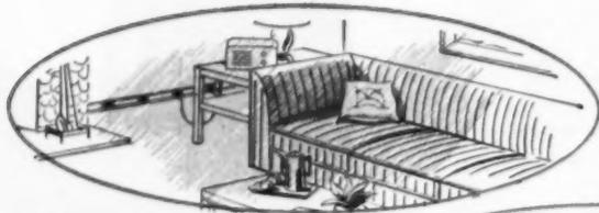
**LIVING ROOM**—Type CF-3 (switch controlled) "Plug-In" Strip provides a complete baseboard of outlets spaced 18" apart. Every outlet provides dual service—switch controlled at doorways or constant service. Allows absolute freedom for furniture rearrangements.
