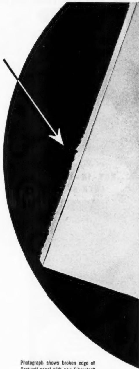
Photograph shows broken edge of Bestwall panel with new Fiberglas\* reinforced gypsum core.
