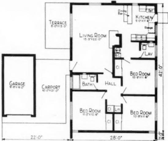
The economical rectangular shape with its uniform wall openings and unbroken roof lines encloses 1,176 square feet of living space, plus 427 square feet more in garage and carport
