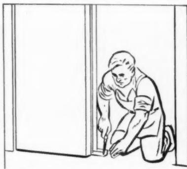
**5** Open doors. Place floor guide halfway under doors, screw to floor. Move doors and secure other side. (55 secs)
