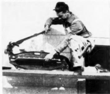
Knife blades are made of high-carbon tool steel, accurately ground and heat-treated. A front-end punch with a fixed gauge for aligning nail holes, and a notching attachment for making all-angle and irregular cuts are standard equipment. Numerous designs, sizes and thicknesses of asbestos shingles can be cut efficiently with this device, the makers say. Specialty Tool Manufacturers, Dept. AB, 732 S. Illinois St., Belleville, Ill.
