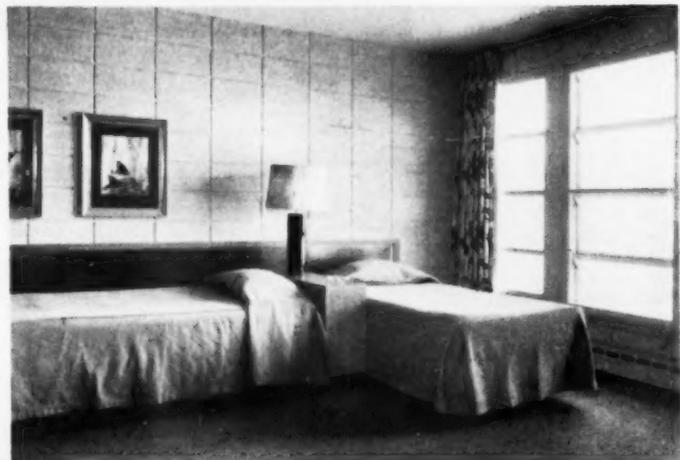
Twin bedroom has studio-type beds. Walls are stacked concrete blocks, painted. Heating is baseboard radiation supplied by boiler located under the office area
