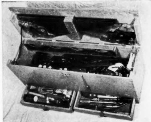
This handy box is a standard item in the equipment of the Henry Bertch company, building contractor in South Pasadena, California. Saws can be removed without breaking their teeth; the level has a place near the
