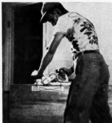
Electric edge-and-surface plane is particularly suitable for fitting doors and for work on other jobs where accurate fitting is required. This 3-inch plane is adjustable during operation with a click lever which makes 1/64-inch adjustments from zero to a maximum of  $\frac{1}{8}$  inch. It bevels right or left at 45 degrees. Reinforced, non-slip cog-belt drive minimizes shock load on the cutter head
