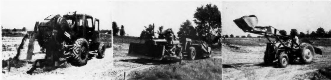
Owned power equipment indispensable to the ABC Construction Corp. operation (l. to r.): trencher, earthmover for subgrade work, high lift for backfilling
