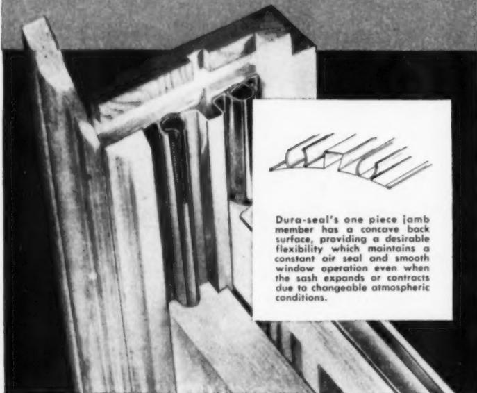
Dura-seal's one piece jamb member has a concave back surface, providing a desirable flexibility which maintains a constant air seal and smooth window operation even when the sash expands or contracts due to changeable atmospheric conditions.
