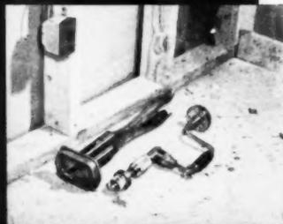
The male cutter snapped in switch box
