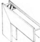
Screw-lock mitted sash corners permit easy re-glazing. ANYBODY can re-glaze a PER-FIT slider sash—in minutes.
