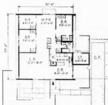
Plan contains 1,395 square feet of floor area and is laid out on a seven foot module. House can be turned in any direction and is designed so carport can be placed on any side
