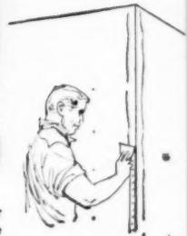
**DUR-A-BEAD**—All-metal, nail-on type outside corner reinforcement for maximum strength and durability; true corners. Finished with PERF-A-TAPE Cement. 8' lengths, packed in 25-piece cartons.
