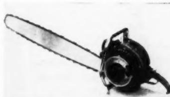
handle; it cuts in any position—up, down or upside down—on all types of cuts, for felling, bucking, boring, notching, trimming or undercutting. Blade sizes include straight blades in 18-, 23-, 30-, 34-, 42-, and 44-inch sizes, and plunge-cut bow saws for one- or two-man operation available in 14- and 18-inch sizes. Homelite Corp., Dept. AB, 111 Riverdale Ave., Port Chester, N. Y.
