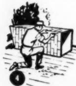
4 Cut housing panels to desired roof ridge or pitch. Assemble with corner angle irons provided.
