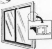
Double Contact Weathering provides flush surface, weather-tight fit.
