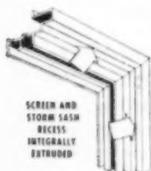
Storm sash and screen hardware are factory located—the actual recess is designed into the frame—no difficult job-condition decisions to make.
