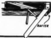
Bevel Bar automatically adjusts itself for all Mitre Cuts on Hip, Valley or Jack Rafters.
