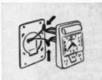
**B.** Connect wires. Operates on 110 v., 60 cy. house current. Outlets rated at 15A.
