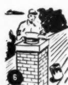
6 Install housing cap. Set chimney pot with joint cement. Rain cap available if needed.
