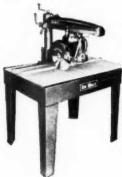
**NEW MODEL GWH—10"** saw, 1 H. P., single phase. Built-in 110-220 volt change switch, cuts 3" deep, rips to center of 48" panel. Legs detach for portable use. Preferred by most small builders. Only \$395 delivered.
