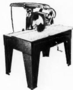
**MODEL R-2K—Retractable arm.** 12" Saw, 2 H. P., single phase. Built-in 110-220 volt change switch. Cuts 3½" deep, rips to center of 65" panel. Big 20" x 1" cut-off capacity—the finest value in the DeWalt line at \$495 F.O.B., Lancaster, Pa. This design has features that outmode all other makes. Also available in 3 and 5 H. P. 14" sizes.
