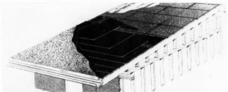
This illustration of built-up roof construction shows roof deck, built-up roofing, granules, gravel stop and gutter
