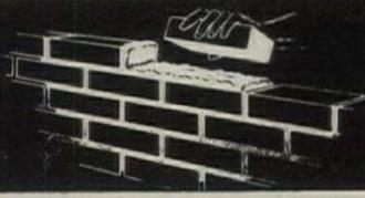
**4 fill mortar joints**... Strong and watertight masonry requires the complete filling of all mortar joints particularly head joints.
