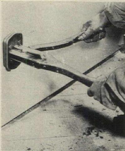
Male and female cutters automatically lock through hole; squeezing handles cuts edges
