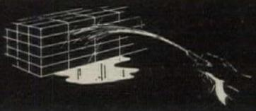
**3 wet units**... High absorption brick and tile should be wet before laying to reduce suction and improve bond between mortar and units.
