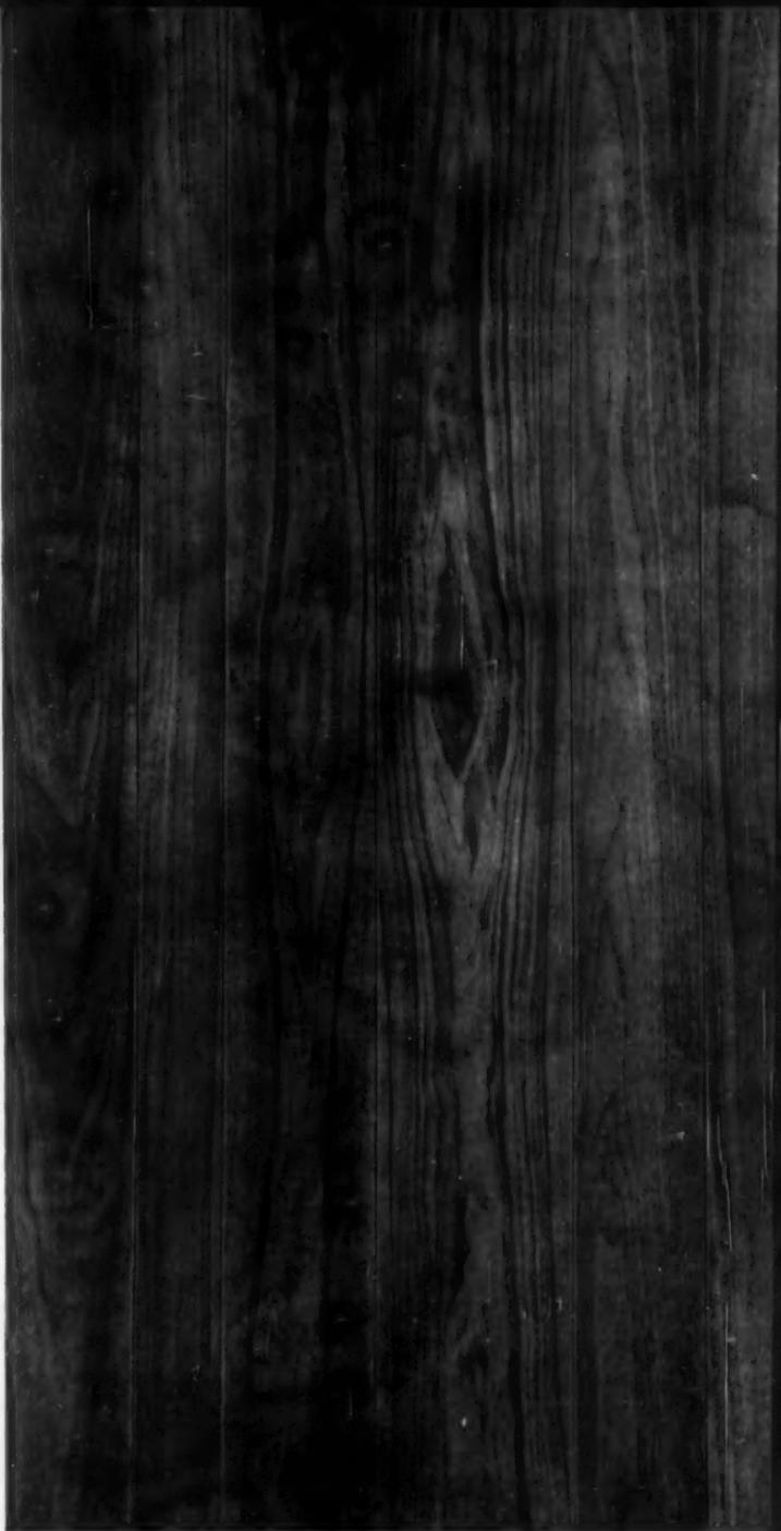
**GROOVES IN V-PLANK WELDWOOD** hardwood panels (4' x 8' x ¼") are spaced like this to give a random paneling effect: 6", 4", 6", 9", 7", 4", 8" and 4". Note that a groove occurs every 16", hiding nails when material is nailed to studs.
