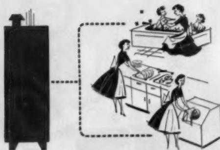
Washing clothes, dishes and the growing American family demands more gallons of hot water per hour, at varying temperatures. Appliances need about 160°, the optimum for 85% of the family wash; the skin takes about 110°. Builders should plan for potential need, with a 40-gallon tank and glass, rock or uncorroding metal linings as requirements. GAMA reports 1,393,500 heaters sold the first half of 1955, 23.3% over the first half of 1954, a trend aided by new shapes and compactness.
