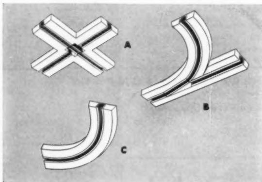
**SPECIAL TRACKS**—PELLA Track Switches and Radial Track enable PELLA DOOR sections to be moved for use or for storage practically anywhere in a room.
