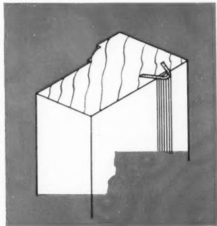
**Vinyl gasket**, shown in drawing dovetails into back face of exterior casing.
