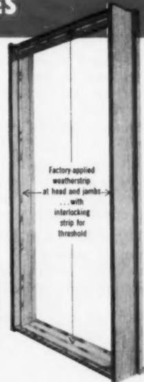
(l to r) Interlocking hook strip. Pine sill reinforced with aluminum extruded strips, the jamb and head, showing aluminum weatherstrip factory-applied to rabbet.
