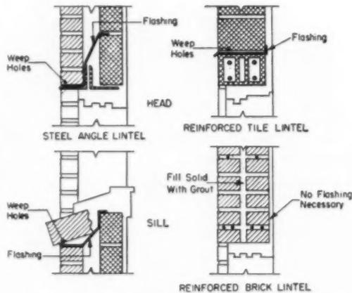
Flashing should be placed under and behind both masonry and wood sills. All heads of openings, except those protected by projecting eaves or hoods, should have through flashing.
