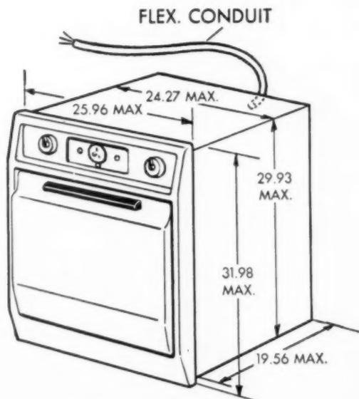
**Same wide 21-inch oven** as General Electric uses for all its ranges. Holds a huge meal. Lined with eye-catching "starlight" grey enamel. Calrod® bake units and "Focused Heat" broiler are enclosed. No old-fashioned open coils.
