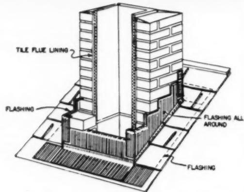
Base flashing of chimneys should extend well back under the roof covering. Counter flashing should be imbedded securely in the mortar joints of the chimney wall.
