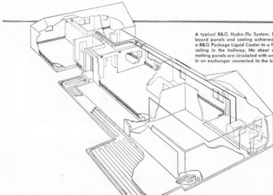
A typical B&G *Hydro-Flo* System. Heat is provided by baseboard panels and cooling achieved by circulating water from a B&G Package Liquid Cooler to a fan-coil unit over a dropped ceiling in the hallway. No sheet metal ducts needed. Snow melting panels are circulated with an anti-freeze solution heated in an exchanger connected to the boiler.
