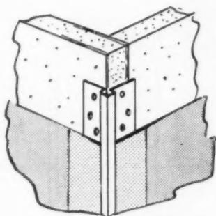
Corner guard for protection to exterior corners applied directly over wallboard and nailed through flange. Nose is undercut to provide grip for spackle finish.
