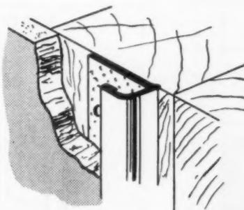
Round or square edge casings are nailed in place before board is applied. Corners are mitered. Inclined plane creates tension that draws board snugly into position.
