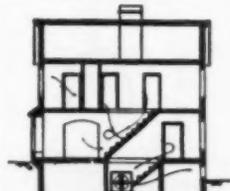
The installation of attic fans generally follows the three methods shown at top of page. In homes with basements it is sometimes practical, and equally effective, to install the fan in a compartment beneath the basement stairs allowing the discharge to exhaust directly into the basement proper. Intake and discharge louvers should follow the same rules that apply to attic installation. The same precautions should be taken against fire.
