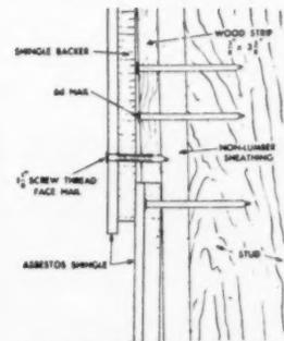
Where insulating or composition sheathing is used wood furring strips provide anchorage for shingles or siding. The latter is face nailed at the bottom only.
