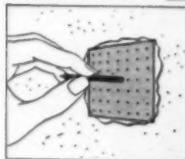
3 Drive Gemco Anchor Nails through furring strips then bend protruding nails over to secure strips.
