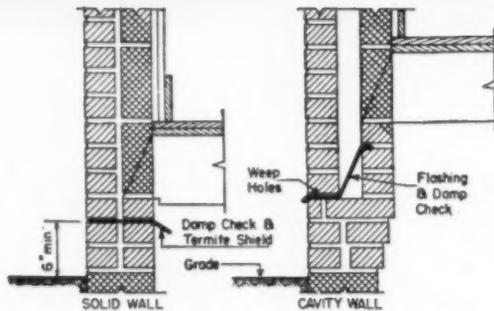
Damp checks should be placed about 6" above grade to prevent moisture, absorbed from the ground by exterior foundations, from traveling upward by capillary action into the wall above.
