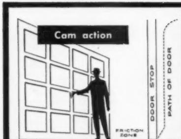
Cam Levers immediately free entire door from stops—friction zone is less than 1/2"!
