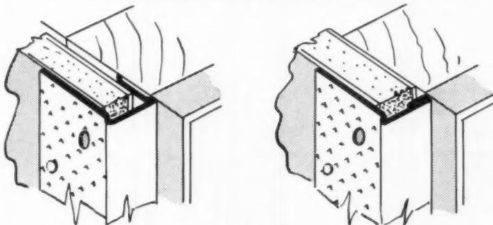
Two types of square edge metal casings which are used to finish edge of wallboard at door jamb or window. Corners are butted and casing is nailed through board into stud. Knurled side affords good spackle adhesion.
