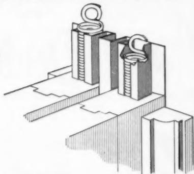
One-piece sash balance and weatherstrip combination unit. A high-quality superior unit, especially designed for PRE-FIT WINDOW UNIT MANUFACTURERS. Ideal for first line-top quality window units.
