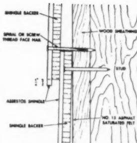
Use of shingle backer where shingles are applied over solid wood sheathing. Shingle backer should be nailed to studs while shingles may be nailed to sheathing.
