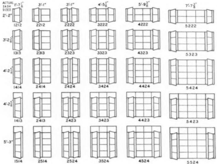
HOPE'S COMBINATION INSIDE-OUTSIDE METAL TRIM is easily and quickly installed with all standard sizes of Hope's Steel Casements. Trim fits into rough openings; no finished carpentry is required, either inside or out. Only a few minutes are needed for assembling at the warehouse or on the job.
