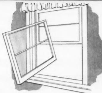
Removable sash hardware. For application with the Master-Matic Unit making a completely balanced, removable sash window.
