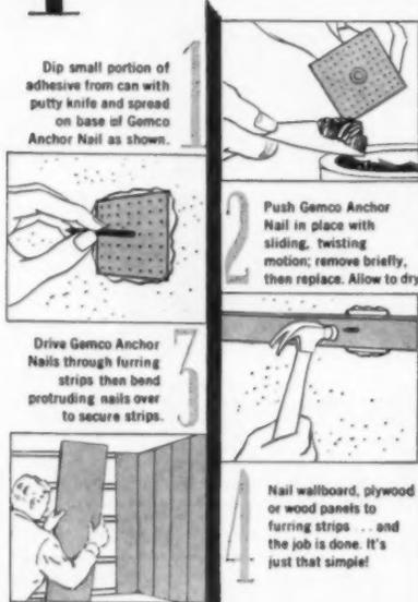
1 Dip small portion of adhesive from can with putty knife and spread on base of Gemco Anchor Nail as shown.
