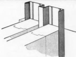
One-piece full jamb liner. A high-quality aluminum weatherstrip unit adaptable for use with ANY TYPE SASH BALANCE, such as spiral, tape, clock spring, etc.
