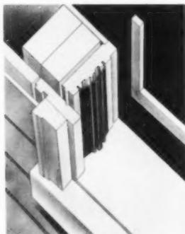
$\frac{25}{32}$ " outside sheathing and dry-wall ( $\frac{3}{8}$ " or  $\frac{1}{2}$ " inside on 2 x 4's, and minus inside strip on jamb.
