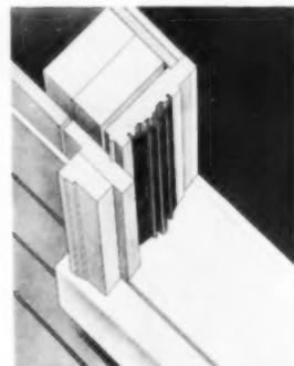
$\frac{1}{2}$ " outside sheathing and  $\frac{3}{8}$ " dry-wall applied over  $\frac{1}{2}$ " insulation board on 2 x 4's, cut-off rib on blind stop.
