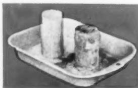
To compare the durability of Brixment with that of ordinary cement-and-lime mortar, make a cylinder or block of each, let both cure for a month or so, then freeze and thaw them about 15 times in your deep-freeze with a little water in the pan.
