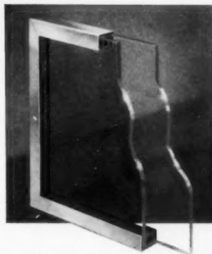
a sealed-in air-space between, giving them their high insulating properties. The entire unit has a stainless steel frame—an exclusive Pittsburgh feature—which protects the seal and glass edges and makes handling quick, safe and easy. Architect: Charles E. Tilton, New York City, N. Y.
