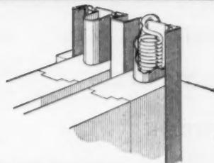
One-piece sash balance and weatherstrip combination economy unit offering all the advantages of the Master-Liner, plus an efficient sash balance. Ideal for low cost-economy window units.
