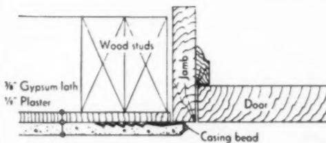
Here,  $\frac{1}{2}$ " casing bead is used over the face of gypsum lath. If gypsum lath laps the bead, a  $\frac{3}{4}$ " depth (with short flange) is used. With metal lath the depth is  $\frac{3}{4}$ ".
