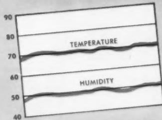
Here's the chart showing Vornado's performance while outside conditions shown above existed. Notice how the temperature remained at an even 70 degrees and humidity never exceeded 50%. Children were running in and out during this extensive test too.
