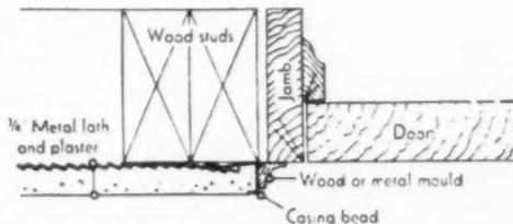
If the door frame is erected after plastering, the casing bead is installed flush with the buck. A small molding closes the joint between buck and frame.
