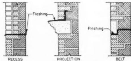
Projections and recesses from the exposed face of the wall tend to hold water or snow and should be flashed, preferably over the top with the outer edge of the flashing bent down and folded as a drip.
