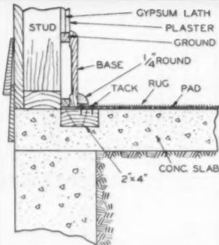
Continuous nailer in concrete slab
