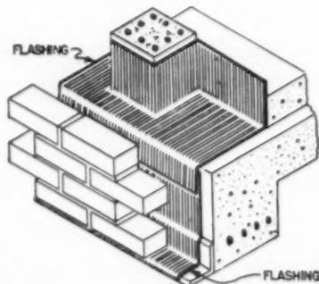
COLUMN & SPANDREL FLASHING
