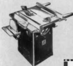
A completely new design concept — safer, easier to use. 8" tilting-arbor saw—4" jointer—10" disc sander. Pays its way on the first job you use it to finish interiors faster, more accurately.
