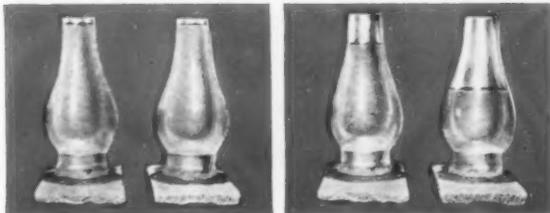
Prepare two slabs of mortar, one with Brixment and one with ordinary cement-and-lime mortar. After mortars have hardened, seal a lamp chimney to each of the mortar slabs, and fill with water.
