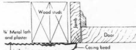
In this detail, the casing bead laps the door frame. Nailing flanges of casing beads have a slight bend to give a spring-tight fit against the frame when nailed in place.
