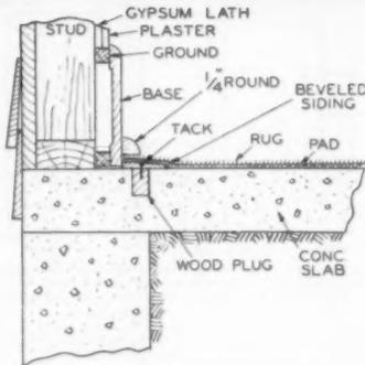
Nailing plugs anchor wood strip
