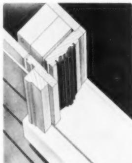
$\frac{25}{32}$ " outside sheathing and  $\frac{3}{4}$ " lath and plaster on 2 x 4's—and full width jamb.
