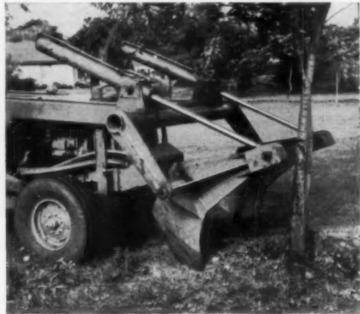
**STARTING TO DIG UP** the tree. See how the bucket shape allows working without damaging the tree trunk.
