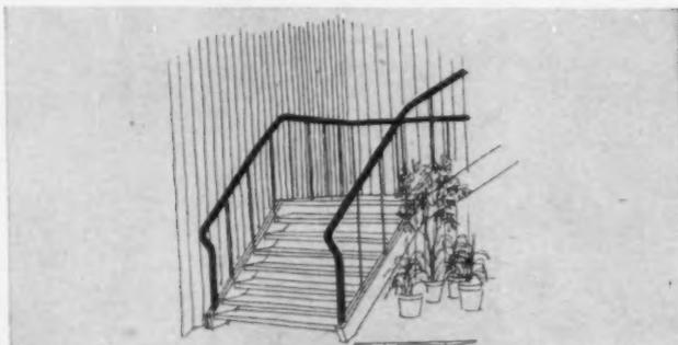
AN INTERESTING STAIRCASE design is achieved by applying vertical siding (thick edge to thick) over 1/4" plywood backing.
