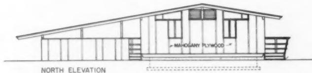
◀ **NORTH ELEVATION** at left. The screened louvers under the gable supply air to the center of house by way of the furred down ceiling.
