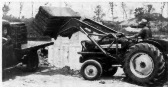
**Utility unlimited!** International 350 Utility gives 1,500-lb capacity with fork lift or half-yard bucket on the heavy-duty front-end loader . . . is easily equipped with rear-mounted fork lift.
