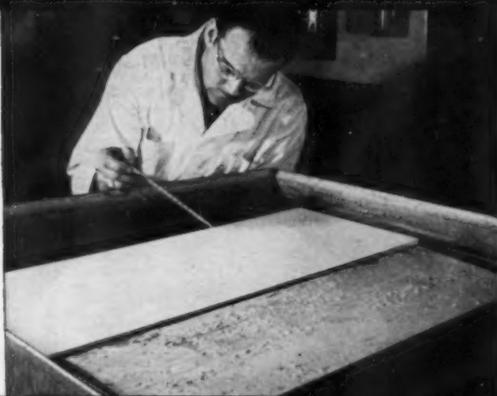
**No more paint blisters?** Experience to date indicates that new Insulite Primed Siding has exceptional resistance to paint blistering. In laboratory test shown above, moisture has bubbled and blistered paint on ordinary siding (in foreground), while Insulite Primed Siding (at back) shows no trace of blistering.
