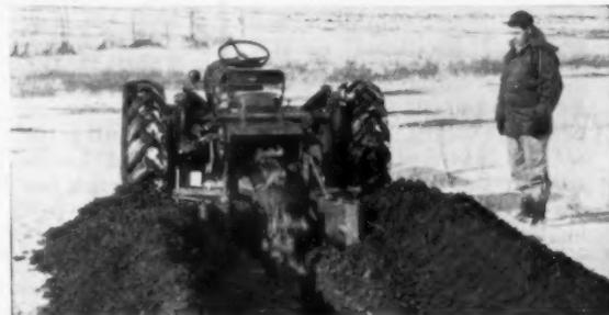
**Trencher digs up to 600 feet per hour**, 5 to 14 inches wide, as deep as 6 feet. Or, dig as deep as 13 feet, 12 to 24 inches wide, with heavy-duty backhoe.
