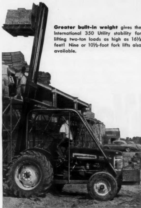
**Greater built-in weight** gives the International 350 Utility stability for lifting two-ton loads as high as 16½ feet! Nine or 10½-foot fork lifts also available.
