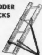
RAIL-TYPE JACK. Use of side rails of ladder for support provides extra safety. Weight, 24 lbs. a pair.
