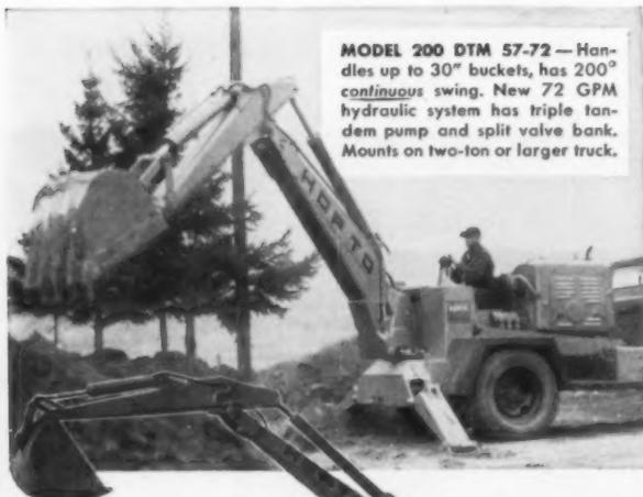
**MODEL 200 DTM 57-72** — Handles up to 30" buckets, has 200° *continuous* swing. New 72 GPM hydraulic system has triple tandem pump and split valve bank. Mounts on two-ton or larger truck.
