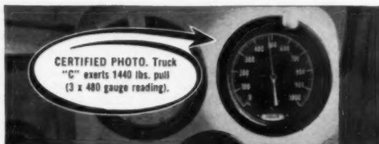
TRUCK C, pulling the same dynamometer truck as the Dodge, was unable to equal the Power Giant mark in repeated tries. Gauges show Dodge outpulled Truck C by 32%.
