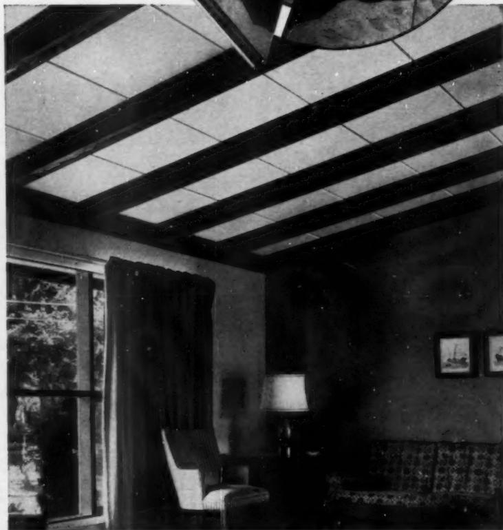
Each Fibretex Panel contains hundreds of small noise traps which absorb up to 75% of the room noise that strikes them. Panels are prefinished in white. Furnished with Lightning Joint or with square edge. Panels are 12" x 12", and 12" x 24", 1/2" and 3/4" thick. All panels come in uniform and random drilled pattern.
