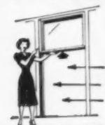
All panels at top — screened ventilation below head level.
