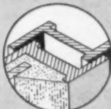
Broad faces of vented sections assure maximum weather protection thru greater metal-to-metal and weatherstripping contact.
