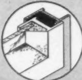
3/16" ventilator web gives greater strength, prevents binding... makes possible tighter closing.
