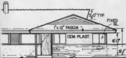
▲ **CONTEMPORARY** exterior: the two-bedroom apartment is part of this unit. Slumpstone masonry, detailed wood paneling and brightly colored stucco add to the modern look. Heavy cedar shake roof has deep overhang.
