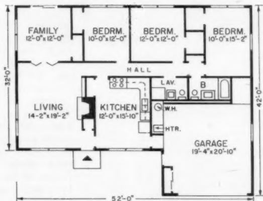
FLOOR PLAN shows how layout is built around baths and kitchen, which in turn are built around garage wall.
