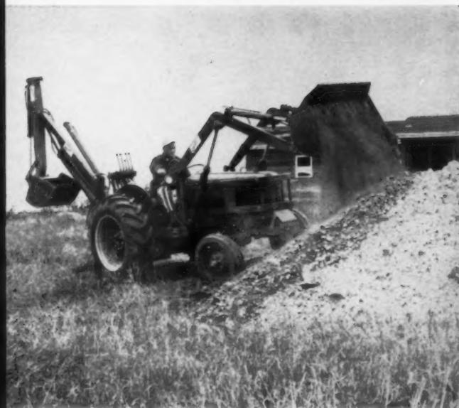
**FRONT-END LOADER** is the other part of the basic tractor rig. Scoop carries more than half a yard, can also be used to scrape and level loose dirt. Many builders use it to dump stone or slag into slab foundations.
