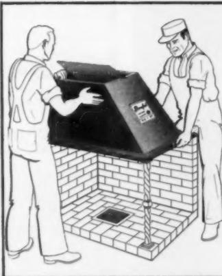
"Just set the Beneform on the brick, on two sides, and on corner post. Since Beneform has three straight sides, it's an easy matter to lay up brick. No lintel bars are necessary. Beneform's flange is 3½" wide, strong enough to carry any load. Masonry is laid right on the flange. No fancy, time-consuming brick-work here."
