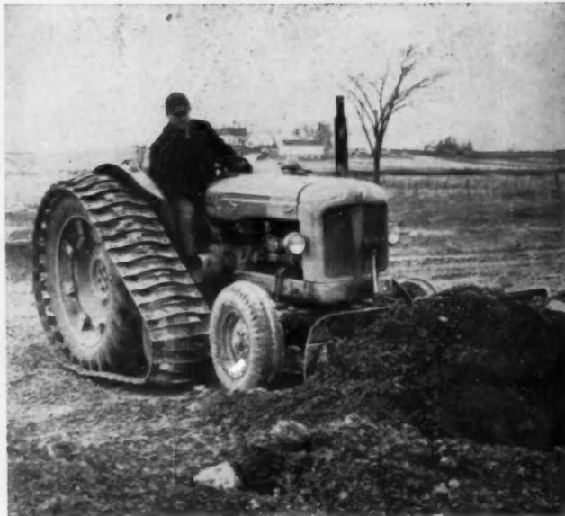
**HALFTRACK ATTACHMENT** by Arps greatly increases traction, makes it possible to use tractor in sloppier ground. While this does not make tractor a bulldozer, it does permit light dozing jobs like the one shown.
