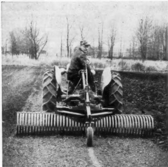
**LANDSCAPING** is one of the biggest jobs done by light tractors. This rake, built by Arps Corp., cleans brush, stones and other debris from area to be seeded. A solid blade can also be mounted on the same frame.
