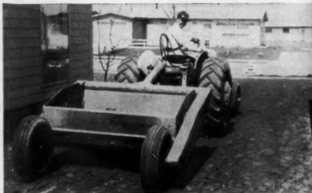
**SMALL PAN**, or scraper, is easily maneuverable, handy for use between houses. It can grade, carry away dirt, or cart it in to fill low spots. And in a pinch, it can truck blocks, bricks, or kegs of nails.
