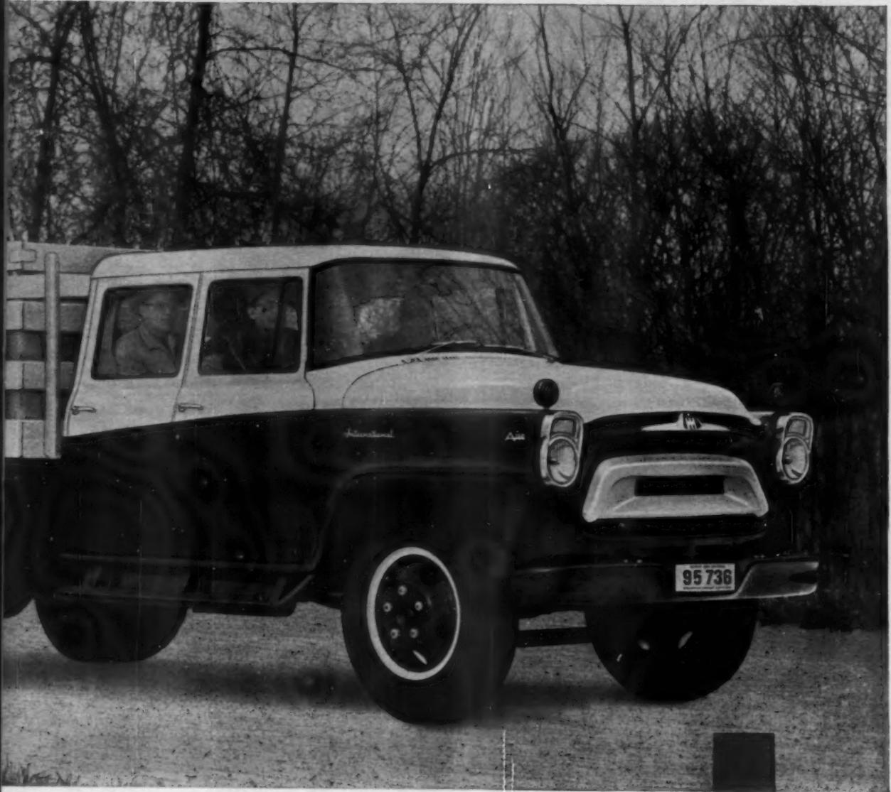
This easy handling INTERNATIONAL model with Travel-Crew cab carries six men in all-weather comfort right to the job site. It's rated up to 25,500 lbs. GVW for heavier loads. Full leg room fore and aft. Seats measure over five feet wide door-to-door. Curbside third door for safer, easier rear entry. Cab and chassis factory-matched. You pay only one low *complete unit* price. Six-cylinder economy, choice of power options. Tandem-axle models to 33,000 lbs. GVW.
