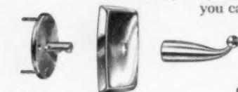
Plate at left is securely attached to wall with screws or toggle bolts, then wall flange is slipped on and held by hook's concealed mounting screw.
