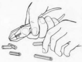
"Hi-RED" anchors may be cut as needed for short screws
