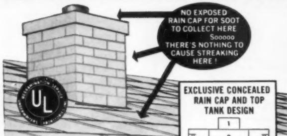
The secret is in the concealed rain cap and top tank design. Vitroliner chimneys have no exposed parts to catch dirty soot that can wash off in the rain and streak the chimney housing or roof. Stainless steel tank collects and evaporates moisture at top preventing it from running down the entire chimney length as in conventional chimneys with bottom "T." No other chimney offers this streak and rainproof protection.
