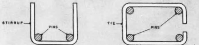
PIN DIAMETER NOT LESS THAN TWO TIMES DIA. OF BAR (FOR STIRRUPS & TIES)
