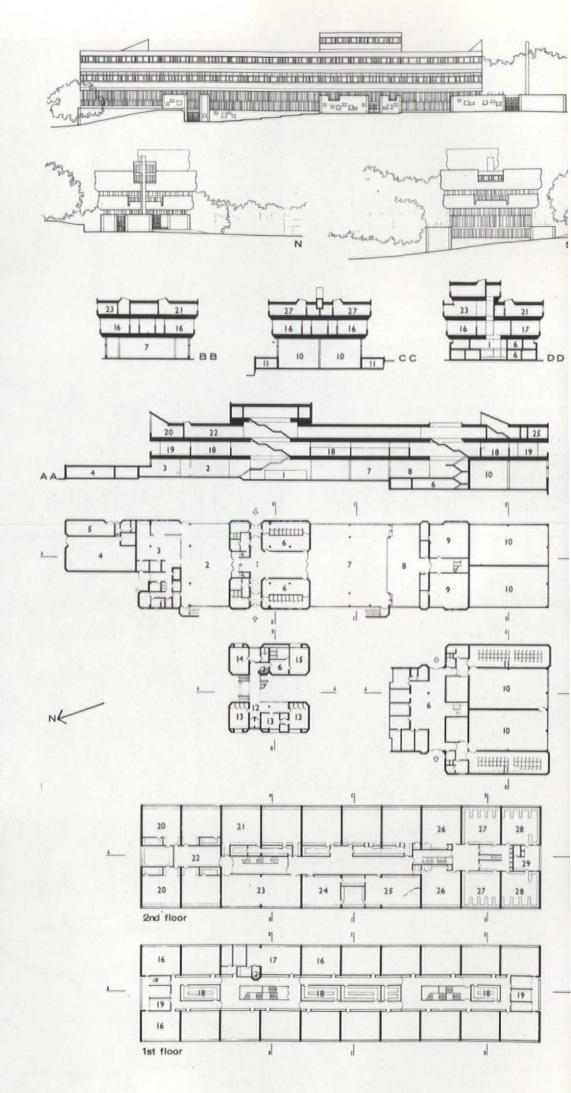
The main appartments on the lower floors are enclosed by a pressed metal, glazed screen with load-bearing rendered brick walls pierced by metal windows in timber sub-frames supporting reinforced concrete floor slabs between.
