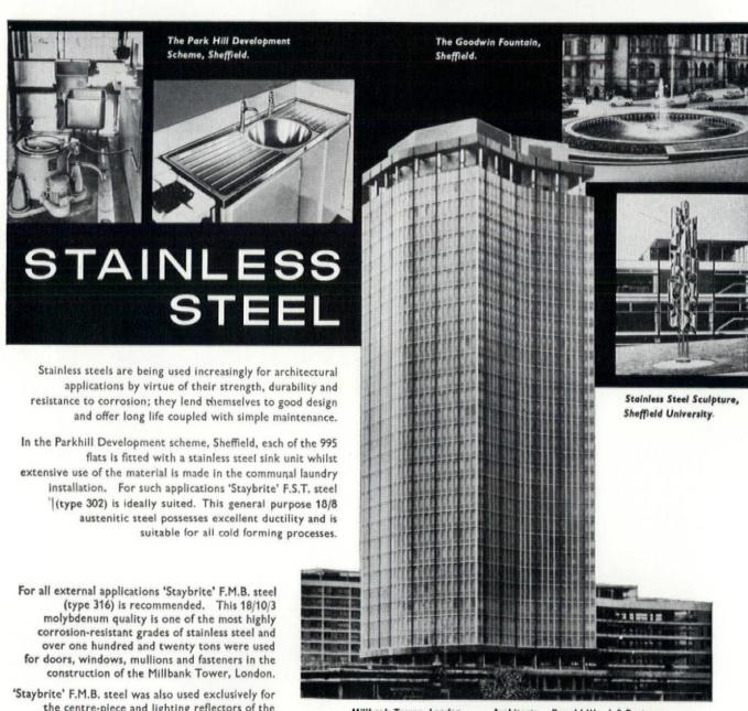
'Staybrite' F.M.B. steel was also used exclusively for the centre-piece and lighting reflectors of the Goodwin Fountain and for the sculpture shown above. This quality is readily weldable by all processes; it is highly ductile and is suitable for rolled or drawn sections and pressed panels of all descriptions. Further information on the use of stainless steels for architecture is obtainable on request.
