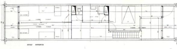
3 Plan at levels, 3, 6, 11 and 14. Plan of typical through apartments
