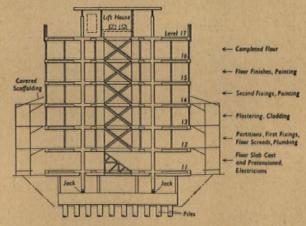
This diagram illustrates the working stages, showing that floors are complete by the time the fourth storey is passed.
