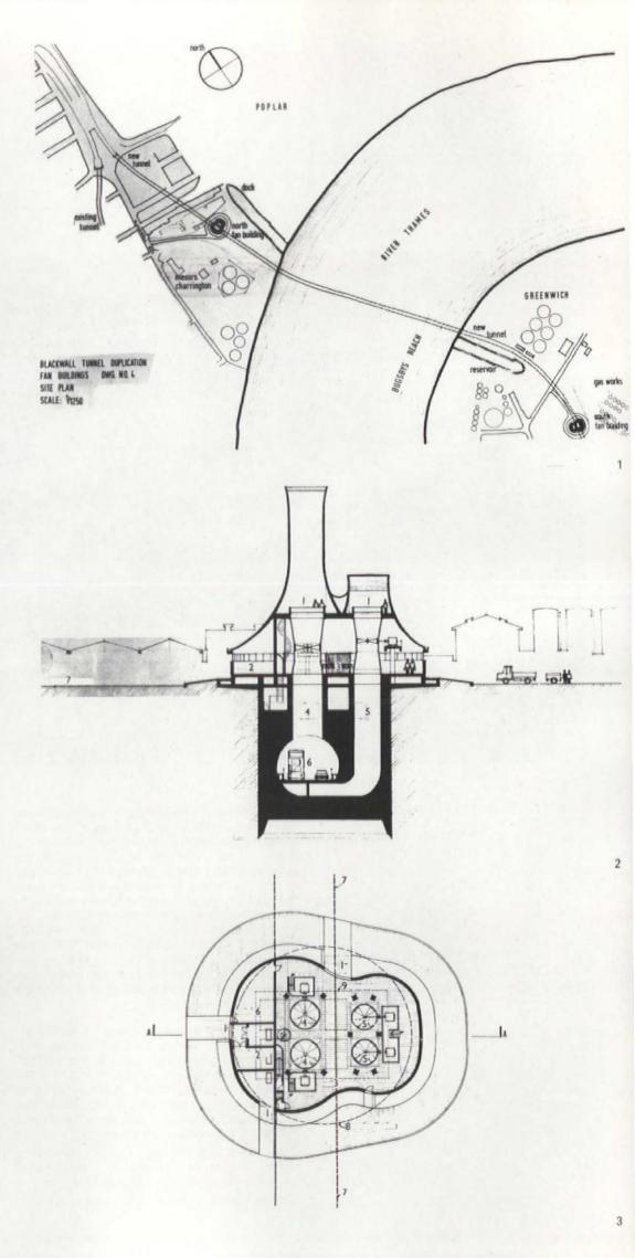
Site plan showing relation of northern and southern fan buildings to the Blackwall tunnel
