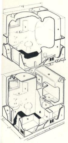
ICI Heart Unit, 1964. Interior surfaces of vacuum formed acrylic sheet moulding reinforced on the exterior with fibreglass-strengthened polyester. The two-storey unit has cloakroom and part of the kitchen below, bathroom above. The moulded frames are enclosed in timber framed plywood panels Key
