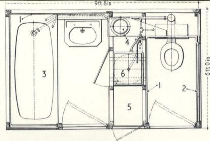
Prefabricated bathroom produced as an exercise for comparison with a typical Local Authority bathroom, costing £240
