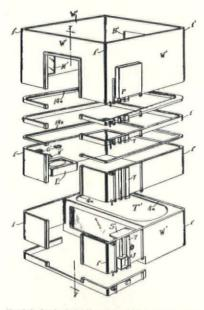
Prefabricated bathroom, USA 1934. An obsessional approach towards integrating of panels and pipes resulting in even greater multiplicity of connections
