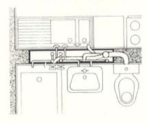
Plumbing assembly by Paul Ramm, Stuttgart. Pipes supplied in a steel angle frame, cast into concrete on site. (FBW)
