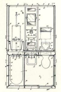
Plan and elevation of a prefabricated bathroom, USA, 1931, in vertical panels. An early attempt to reduce plumbing costs. Number of plumbing connections same as for normal site assembly
