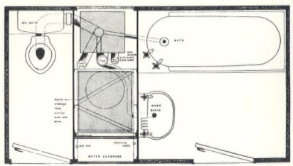
Arcon bathroom unit 1964. Designed for a Ministry of Housing 5M pilot scheme in Sheffield. 10ft 8in  $\times$  6ft 0in based on a 4in module. Weight 1 $\frac{1}{4}$ tons. Frame of cold rolled steel sections with floor and wall sections bolted on. Skeleton timber frame faced with  $\frac{1}{4}$ in hardboard or plywood. Supplied with steel lifting tackle and jig. Offloading time claimed to be three minutes; and connection of four services, 45 minutes
