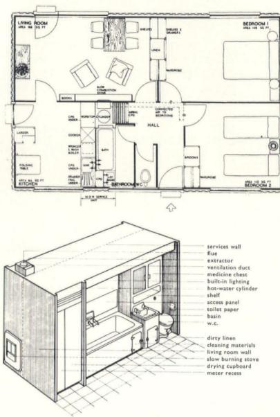
Arcon house plan and MoW mechanical core (FBW)
