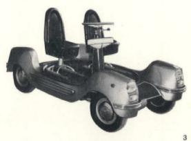
1, 2 & 3 Urbanina—a small Italian car designed by the Marquis Piergirolamo and the engineer Narciso Cristiani to reduce the amount of space occupied as much as possible. The two-seater body swivels on a circular turntable independently of the wheelbase, so that the driver and passenger can get out on any side.
