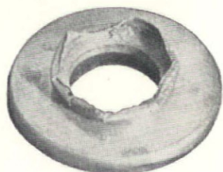
Abrasive damage to handle bearing subjected to dry friction, a defect now usually eliminated by the use of nylon bushes or, in the case of Wehag handles, by an absorbent bearing ring of sinter metal
